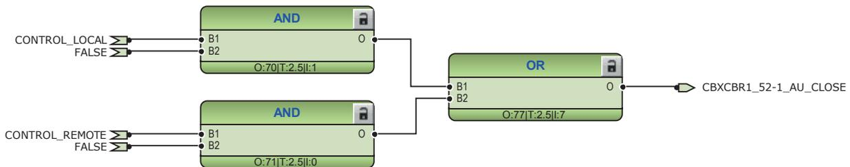
Figure 147: External closing command for circuit breaker
