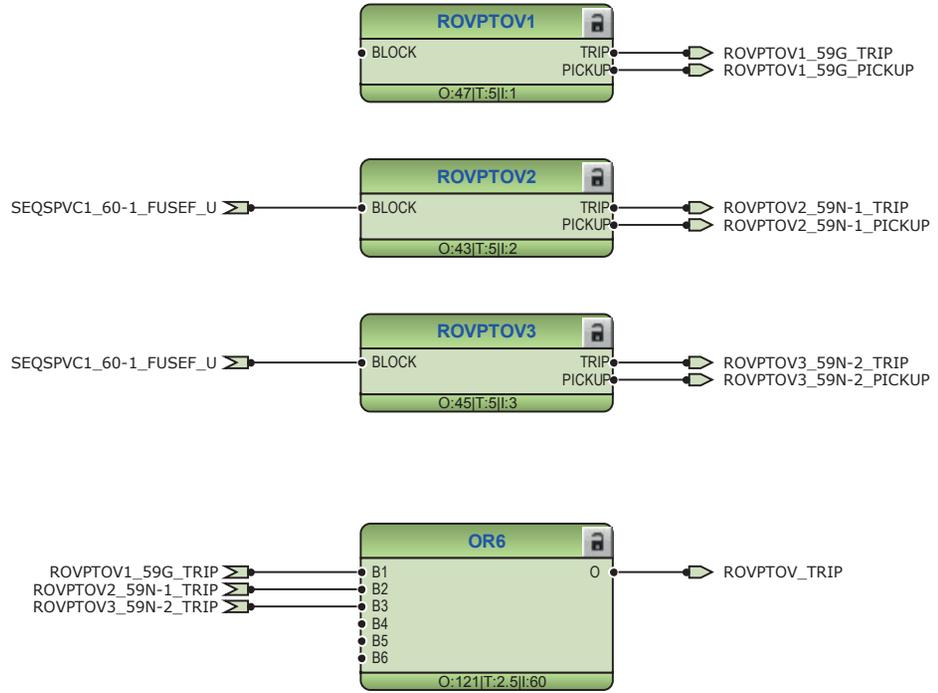
Figure 186: Residual voltage protection function
