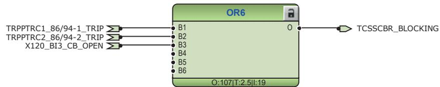
Figure 198: Logic for blocking of trip circuit supervision
