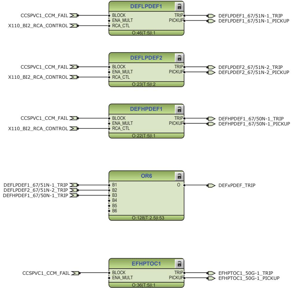
Figure 58: Non-directional ground-fault protection
