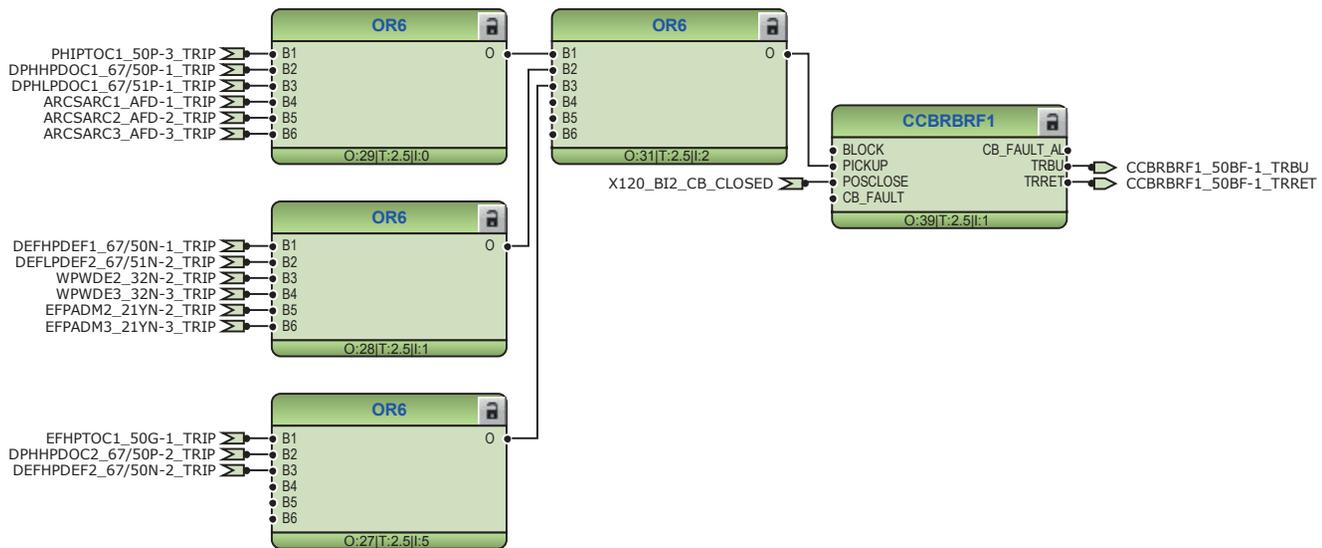
Figure 179: Circuit breaker failure protection function
