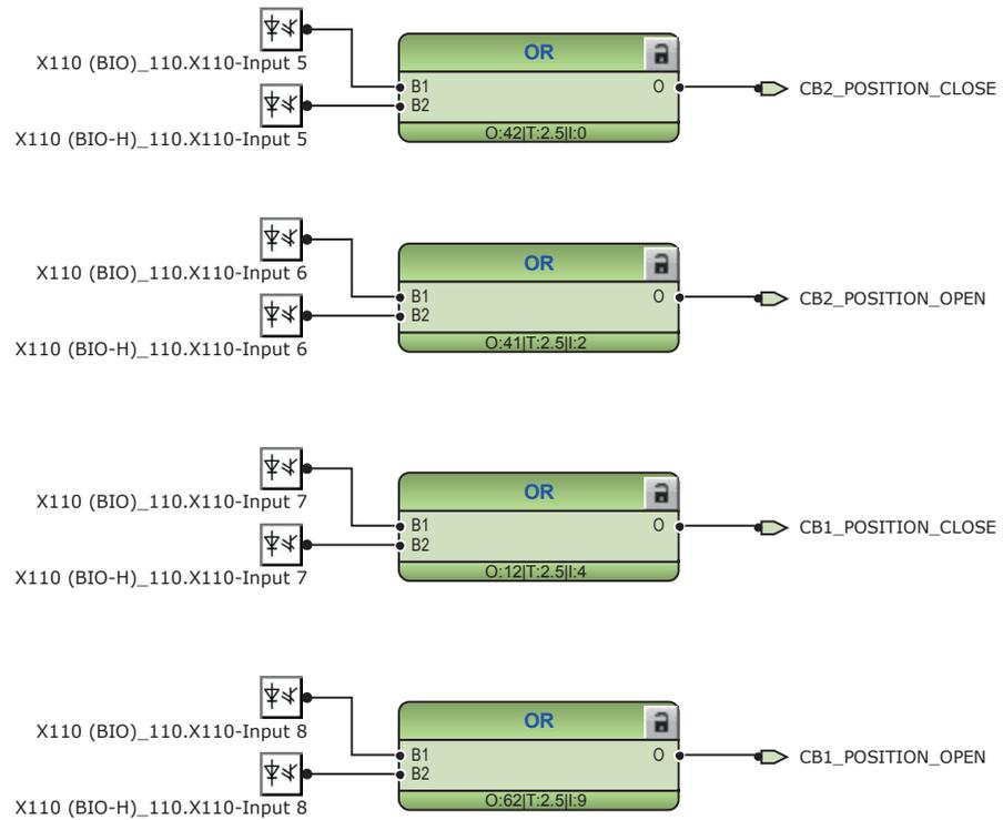
Figure 248: Default binary inputs - X110
