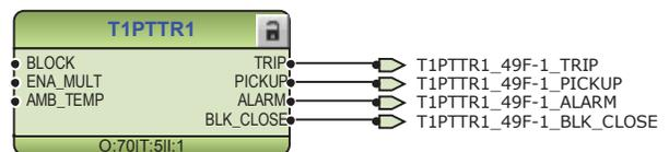
Figure 63: Thermal overcurrent protection function
