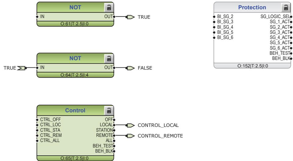
Figure 162: Functions for general logic states TRUE and FALSE, protection setting group selection and local and remote control
