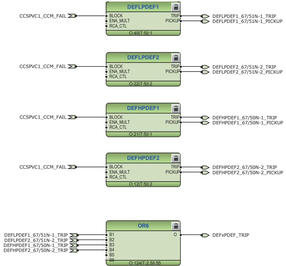
Figure 115: Directional Ground fault protection function
