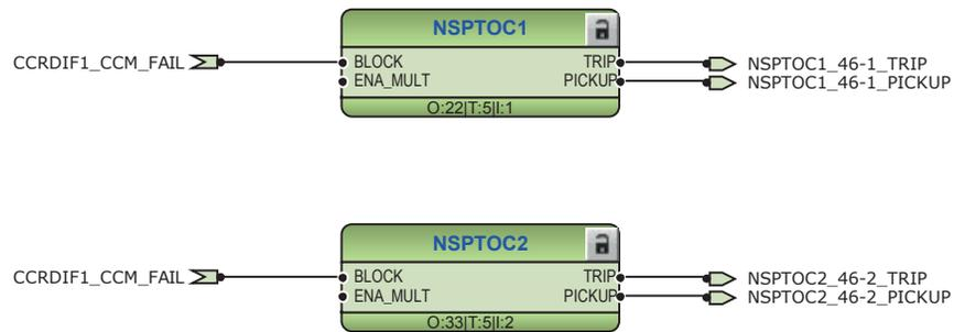
Figure 230: Negative-sequence overcurrent protection
