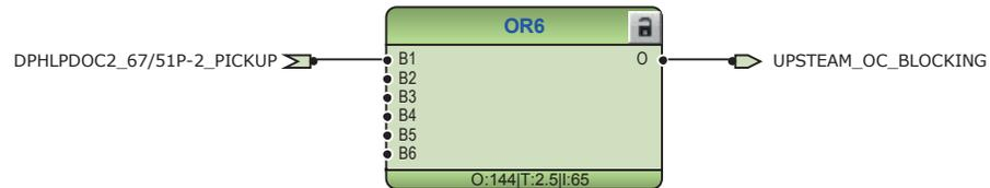
Figure 169: Upstream blocking logic
