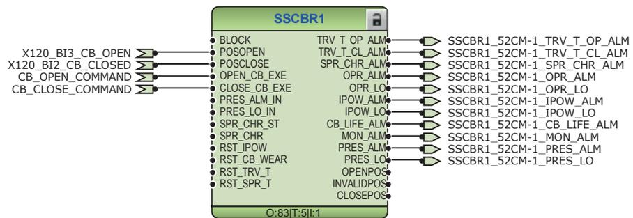
Figure 195: Circuit-breaker condition monitoring function
