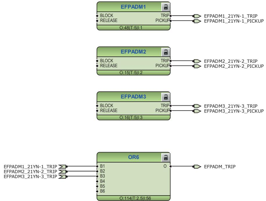
Figure 176: Admittance-based ground-fault protection function
