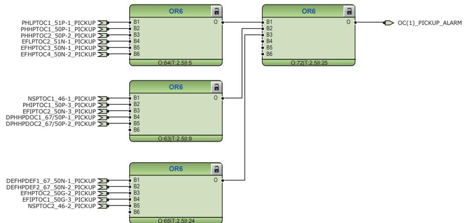
Figure 231: Overcurrent pickup alarm
