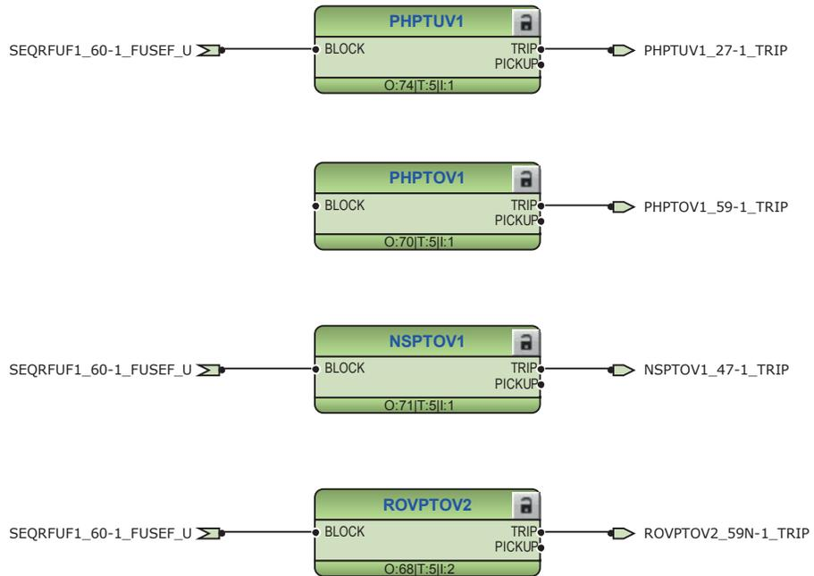
Figure 232: Voltage functions on bus 1
