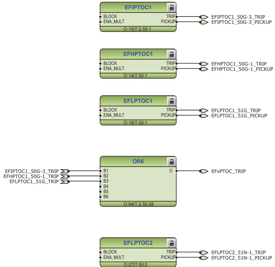
Figure 19: Non-directional ground-fault protection
