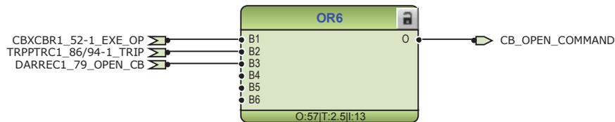
Figure 36: Circuit breaker control logic: Signals for the opening coil of circuit breaker 1
