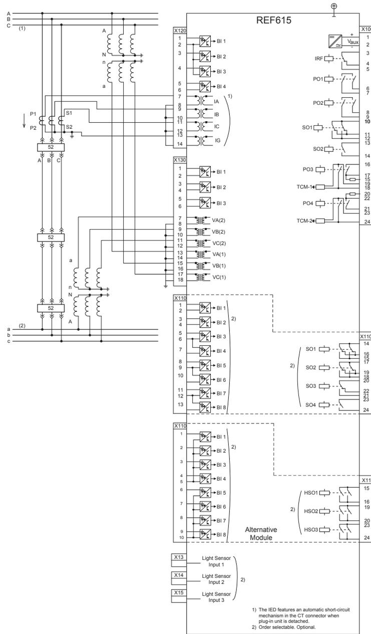
Figure 13: Connection diagram for the P configuration
