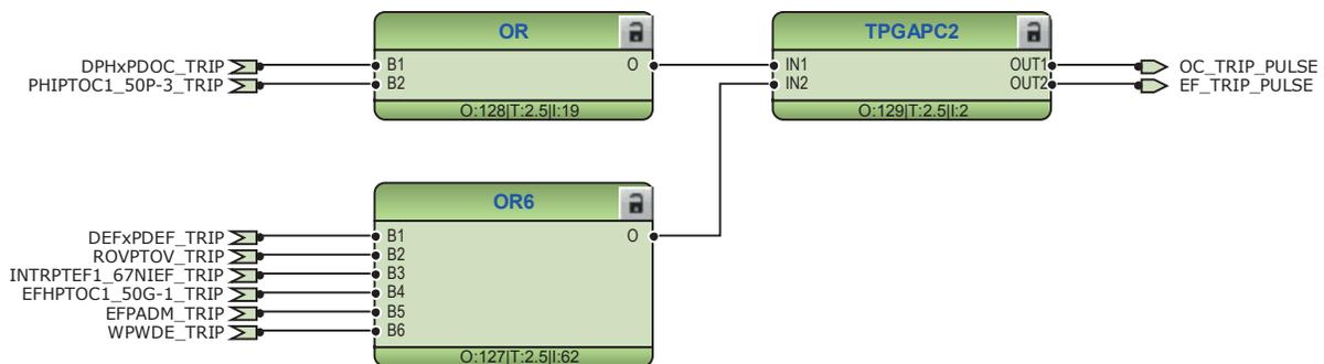
Figure 163: Timer logic for overcurrent and ground-fault trip pulse
