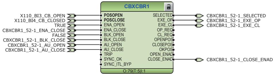
Figure 142: Circuit breaker control logic: Circuit breaker 1
