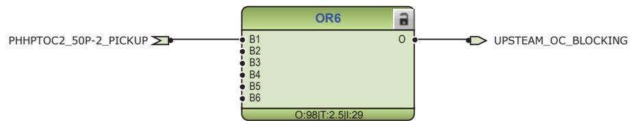
Figure 16: Upstream blocking logic
