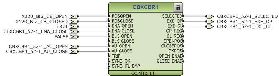
Figure 34: Circuit breaker control logic: Circuit breaker 1
