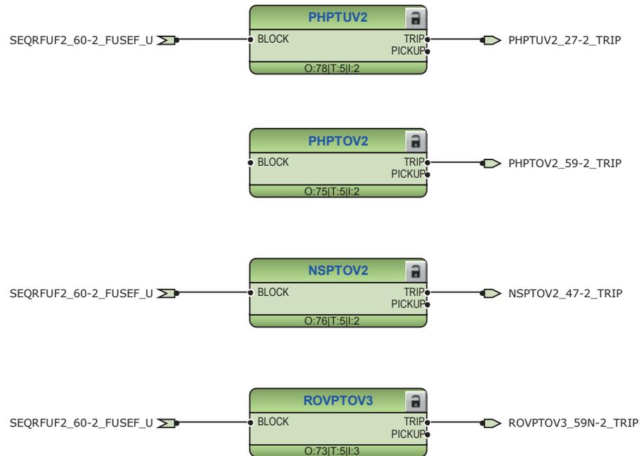
Figure 233: Voltage functions on bus 2
