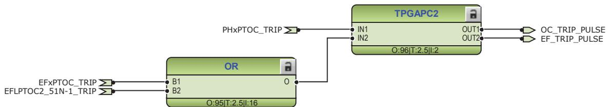
Figure 50: Timer logic for overcurrent and ground-fault trip pulse
