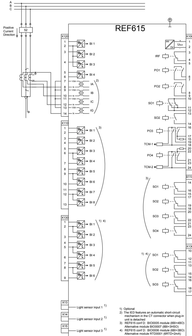
Figure 9: Connection diagram for the D configuration
