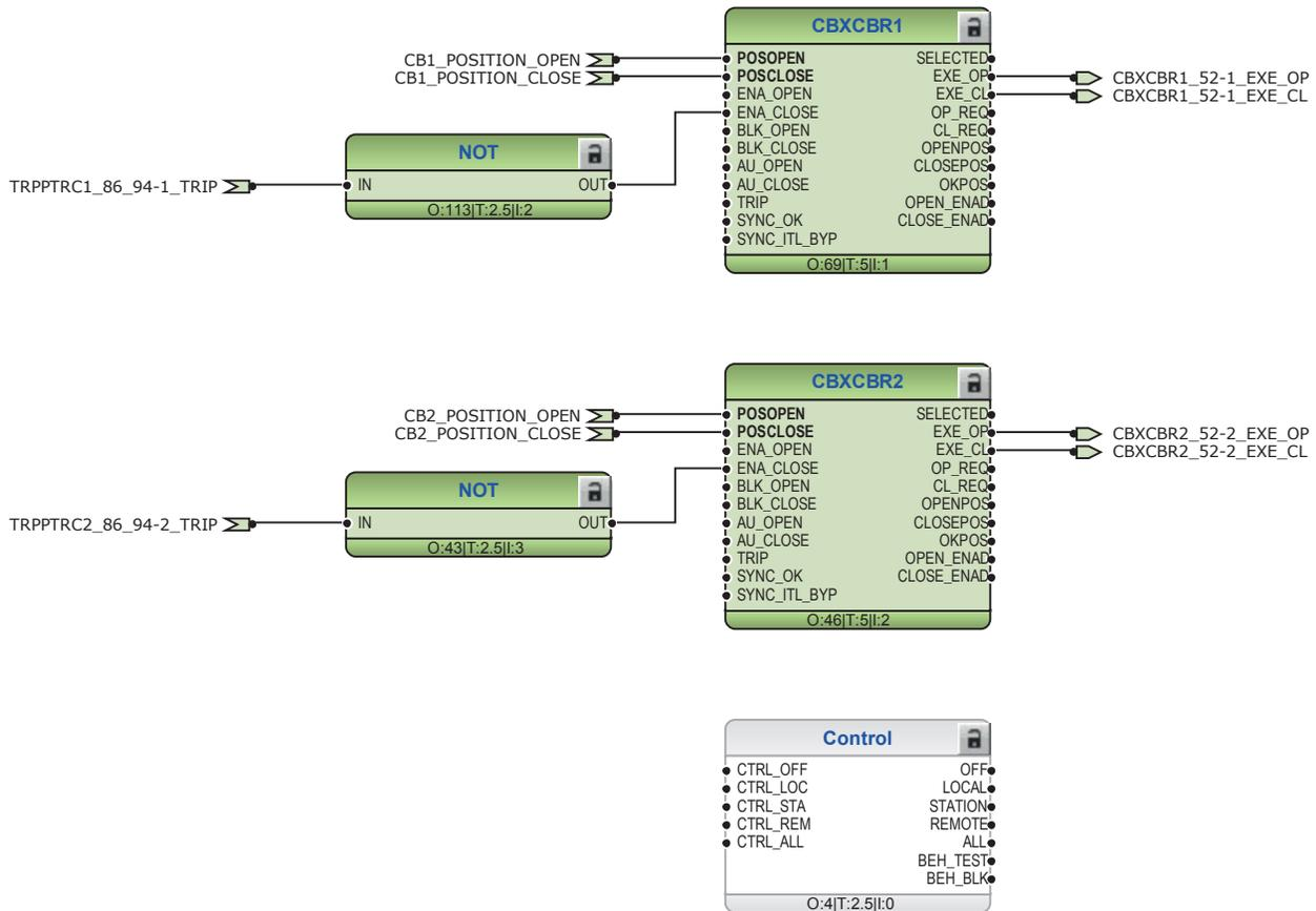
Figure 244: Circuit breaker control
