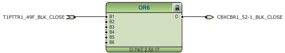
Figure 149: Circuit breaker 1 close blocking logic
