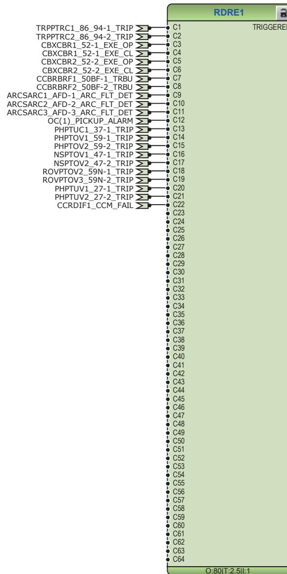
Figure 238: Disturbance recorder
