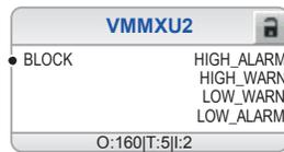
Figure 209: Three-phase voltage measurement
