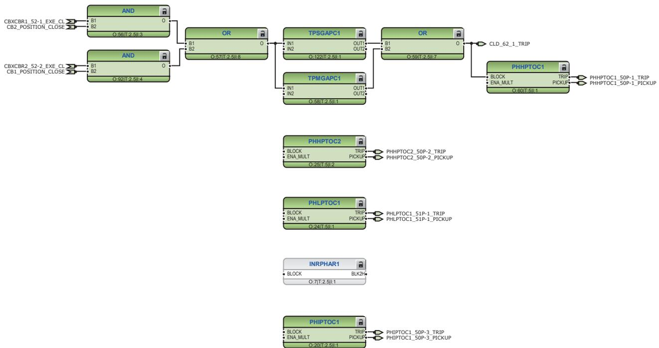
Figure 225: Three-phase overcurrent protection
