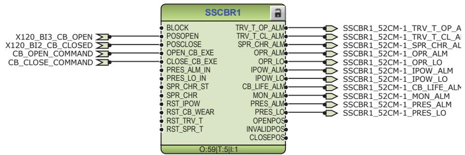
Figure 30: Circuit-breaker condition monitoring function
