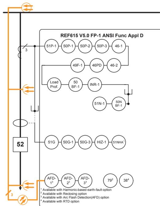
Figure 14: Functionality overview for standard configuration D
