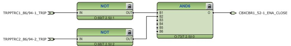
Figure 202: Circuit breaker close enable logic
