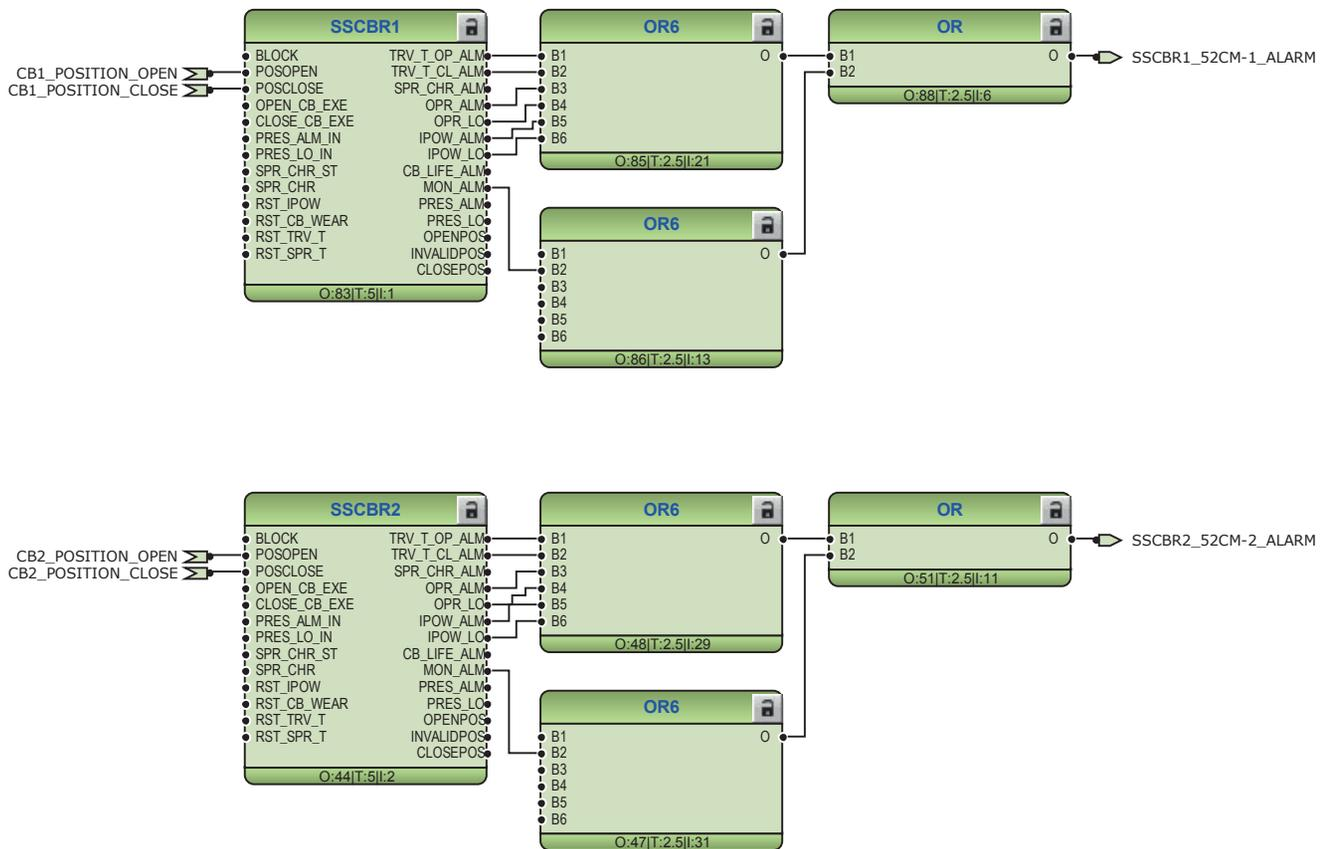
Figure 240: Circuit breaker condition monitoring
