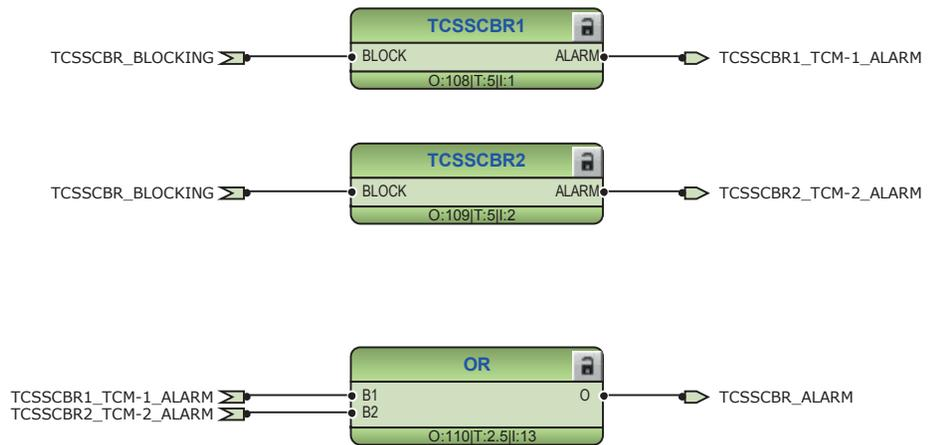
Figure 197: Trip circuit supervision function
