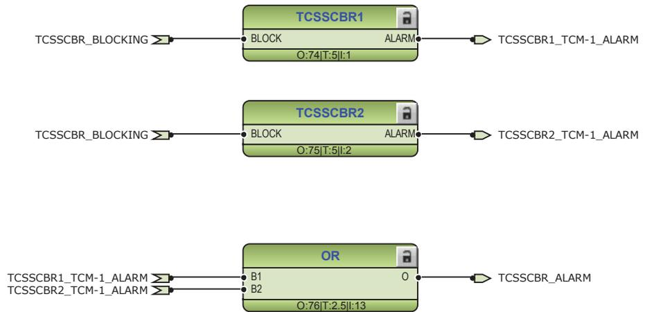
Figure 32: Trip circuit supervision function
