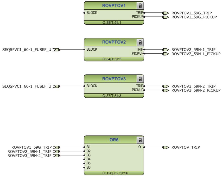
Figure 71: Residual voltage protection function
