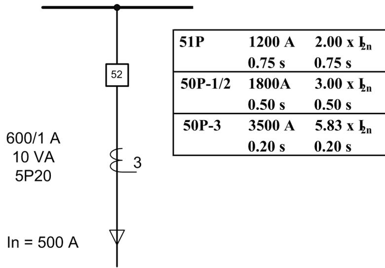
Figure 254: Example of three-stage overcurrent protection
