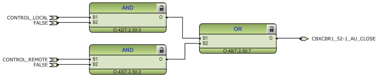
Figure 38: External closing command for circuit breaker
