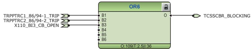
Figure 140: Logic for blocking of trip circuit supervision
