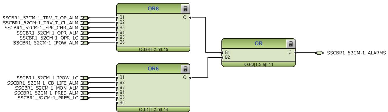
Figure 31: Logic for circuit breaker monitoring alarm
