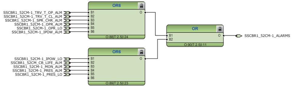
Figure 138: Logic for circuit breaker monitoring alarm
