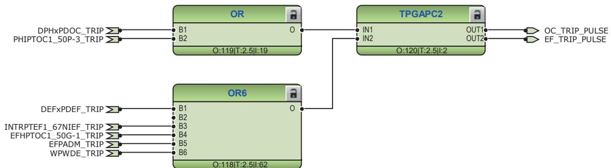
Figure 221: Timer logic for overcurrent and ground-fault trip pulse
