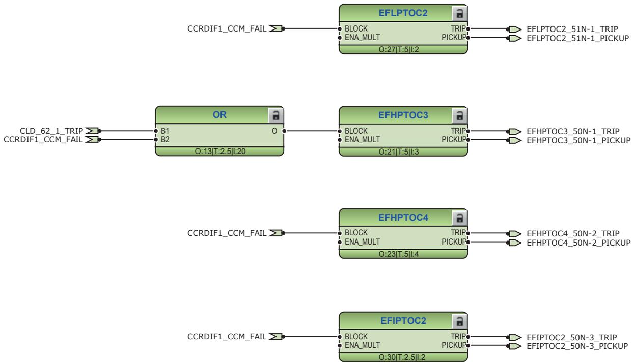
Figure 227: Non-directional calculated neutral overcurrent protection
