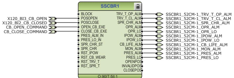
Figure 79: Circuit-breaker condition monitoring function
