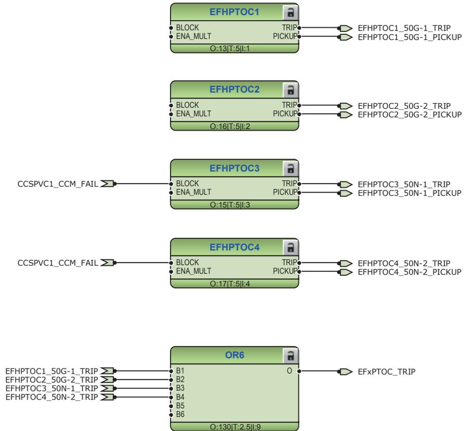
Figure 114: Ground fault protection function
