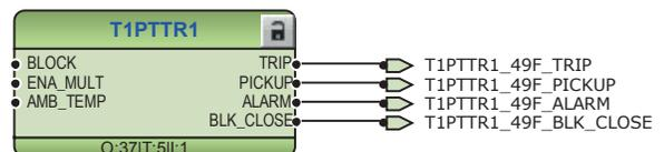
Figure 120: Thermal overcurrent protection function
