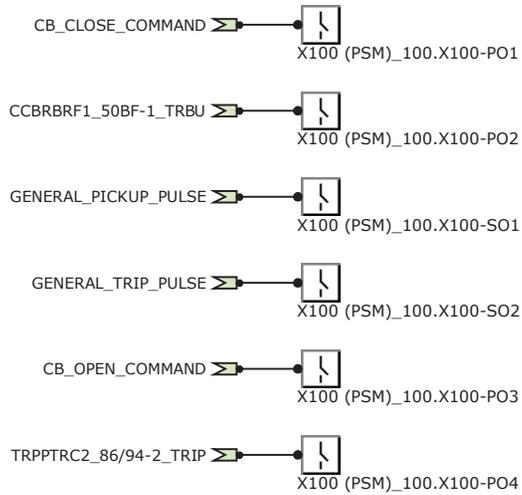
Figure 160: Default binary outputs - X100 terminal block
