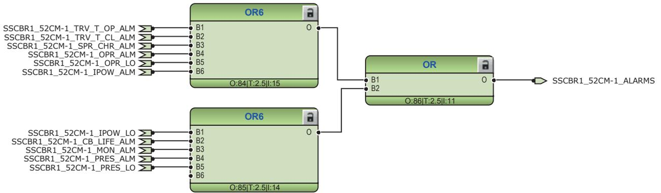
Figure 196: Logic for circuit breaker monitoring alarm
