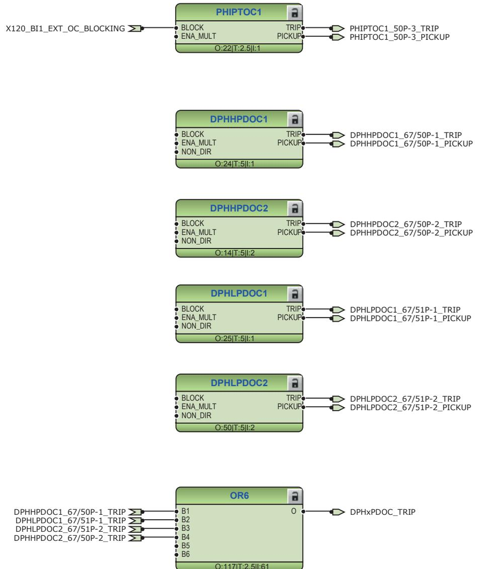
Figure 168: Overcurrent protection functions
