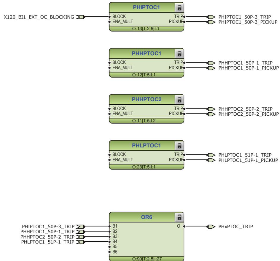
Figure 15: Overcurrent protection functions
