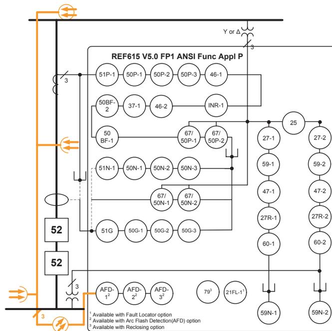
Figure 224: Functionality overview for standard configuration P
