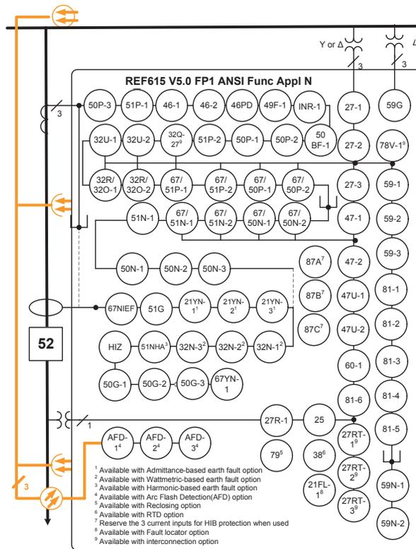
Figure 167: Functionality overview for standard configuration N
