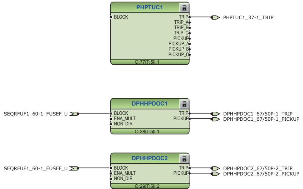
Figure 226: Under current and directional overcurrent protections
