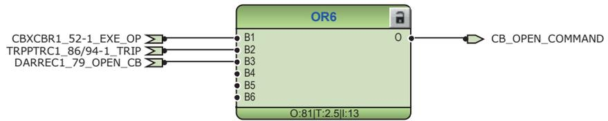
Figure 201: Circuit breaker control logic: Signals for the opening coil of circuit breaker 1
