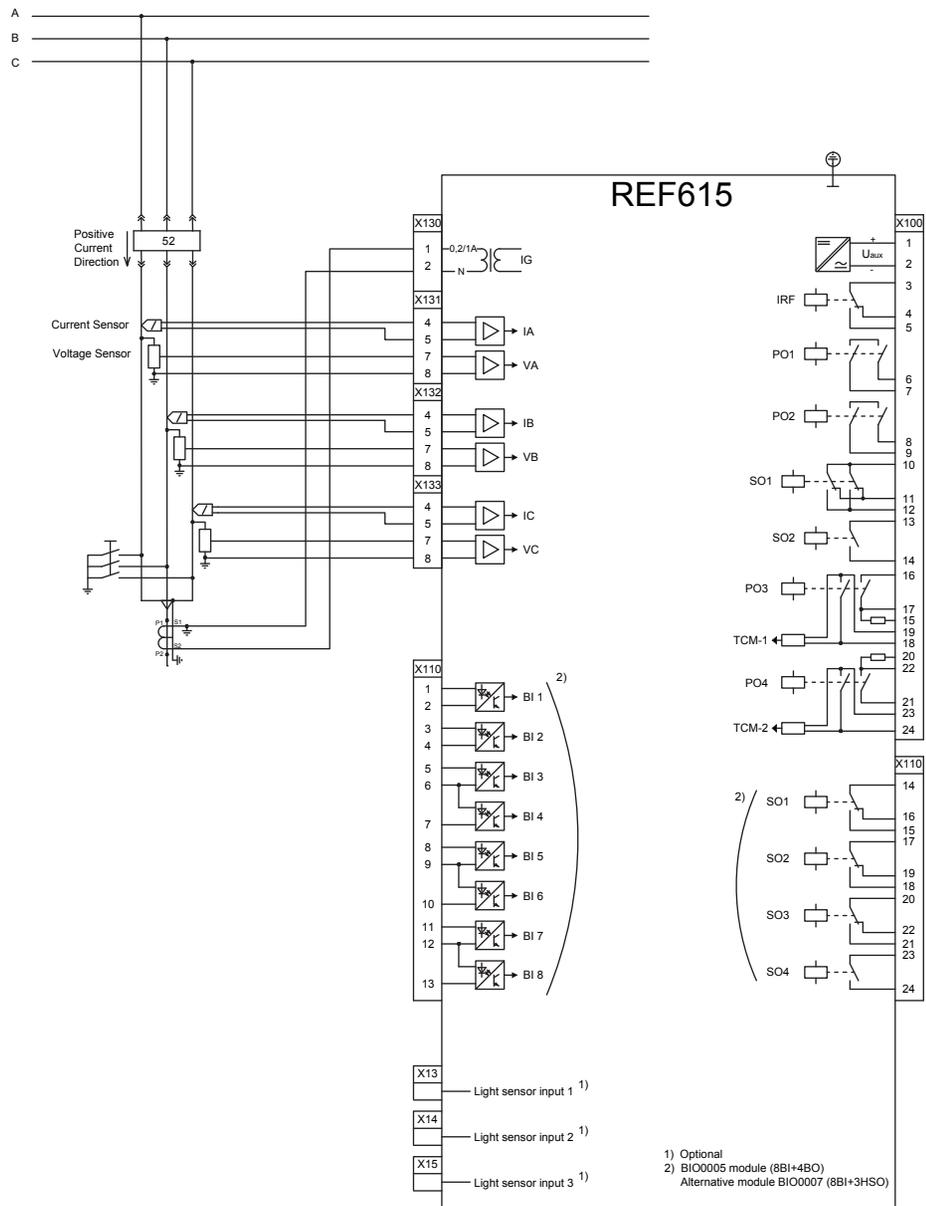
Figure 11: Connection diagram for the L configuration
