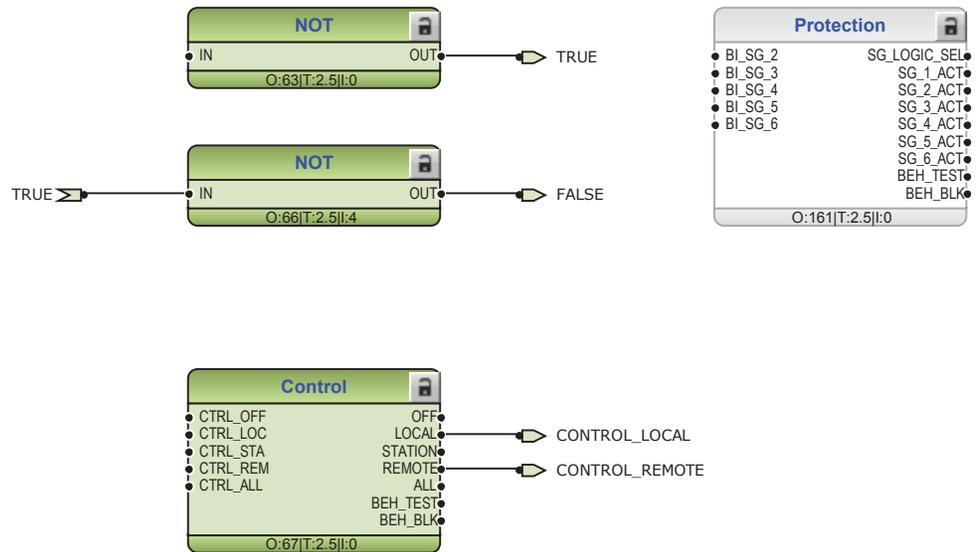
Figure 104: Functions for general logic states TRUE and FALSE, protection setting group selection and local and remote control
