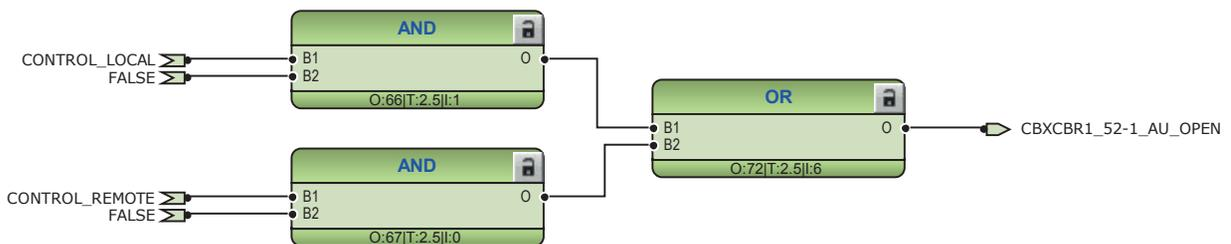
Figure 204: External opening command for circuit breaker
