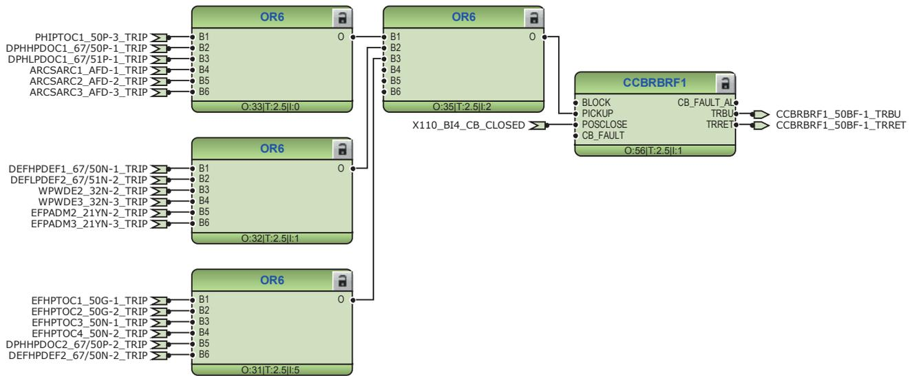
Figure 121: Circuit breaker failure protection function
