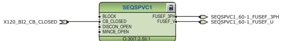
Figure 194: Fuse failure supervision function
