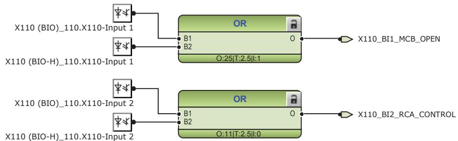
Figure 99: Default binary inputs - X110
