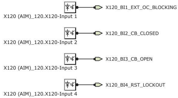
Figure 218: Default binary inputs - X120
