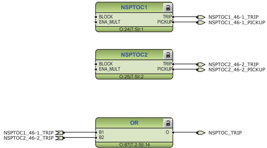
Figure 18: Negative-sequence overcurrent protection function
