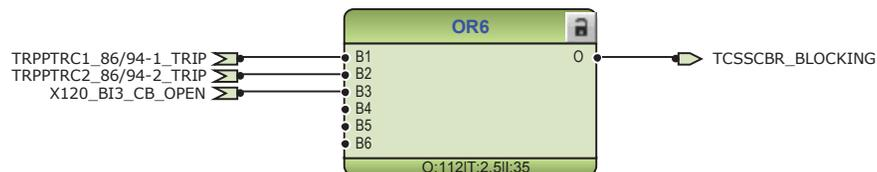
Figure 82: Logic for blocking of trip circuit supervision
