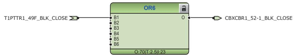
Figure 205: Circuit breaker 1 close blocking logic
