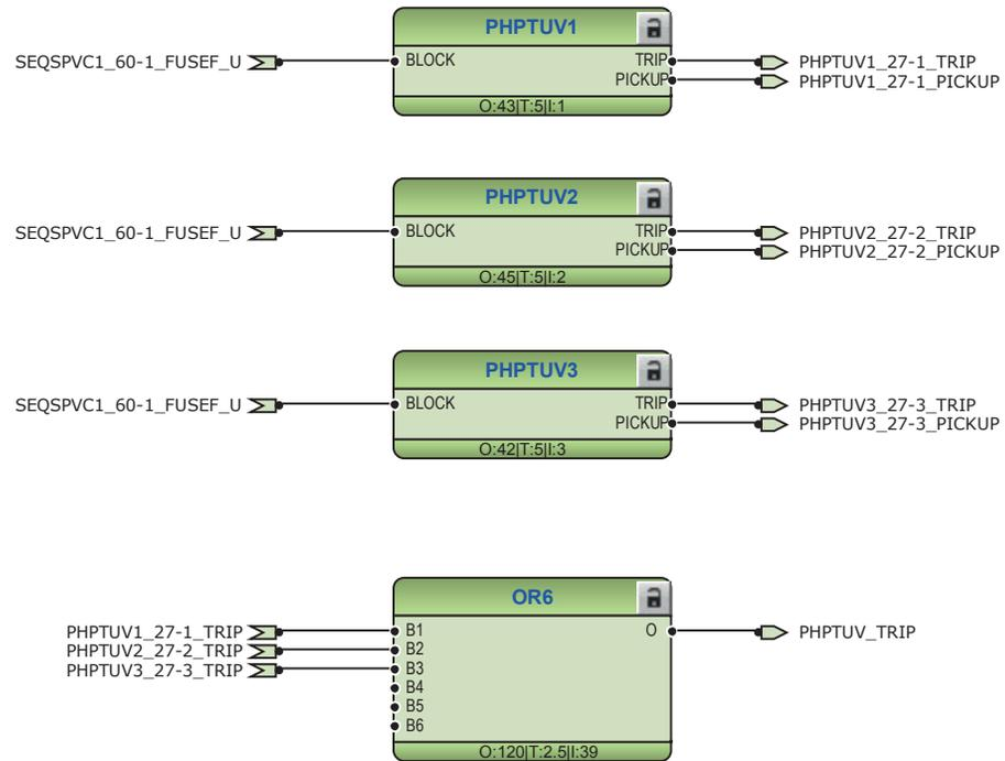
Figure 125: Undervoltage protection function
