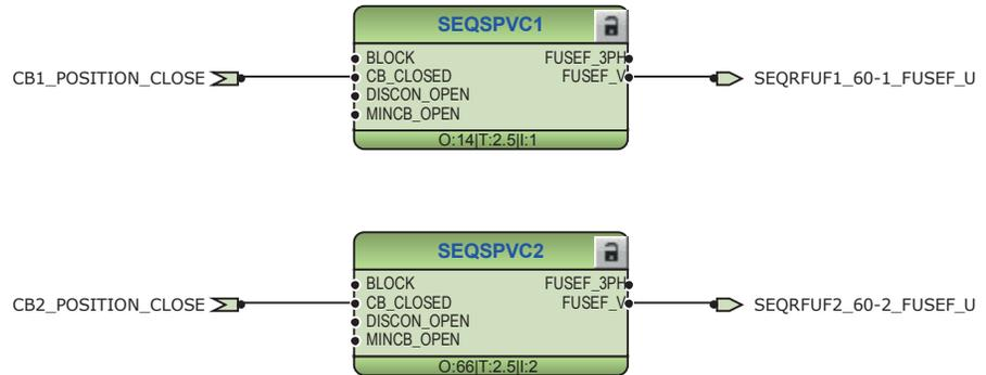
Figure 242: Fuse failure monitoring
