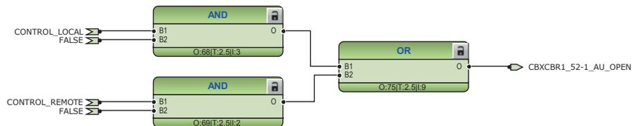
Figure 148: External opening command for circuit breaker
