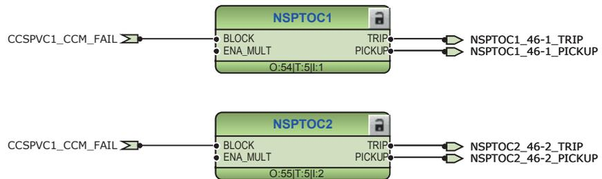
Figure 113: Negative-sequence overcurrent protection function
