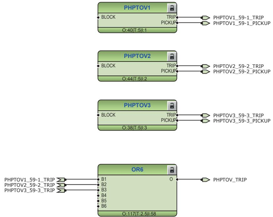
Figure 124: Overvoltage protection function
