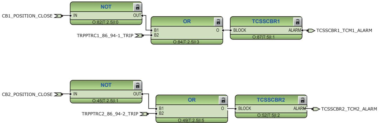
Figure 239: Trip circuit monitoring
