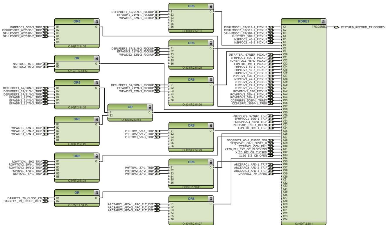
Figure 76: Disturbance recorder
