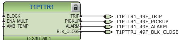
Figure 178: Thermal overcurrent protection function
