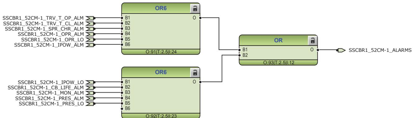
Figure 80: Logic for circuit breaker monitoring alarm
