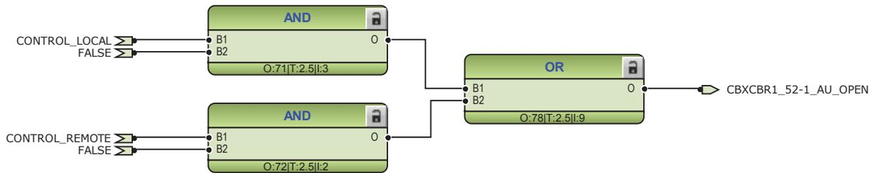
Figure 88: External opening command for circuit breaker
