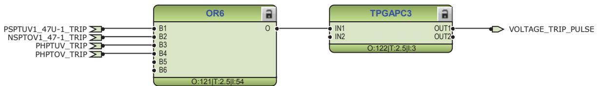
Figure 106: Timer logic for voltage trip pulse
