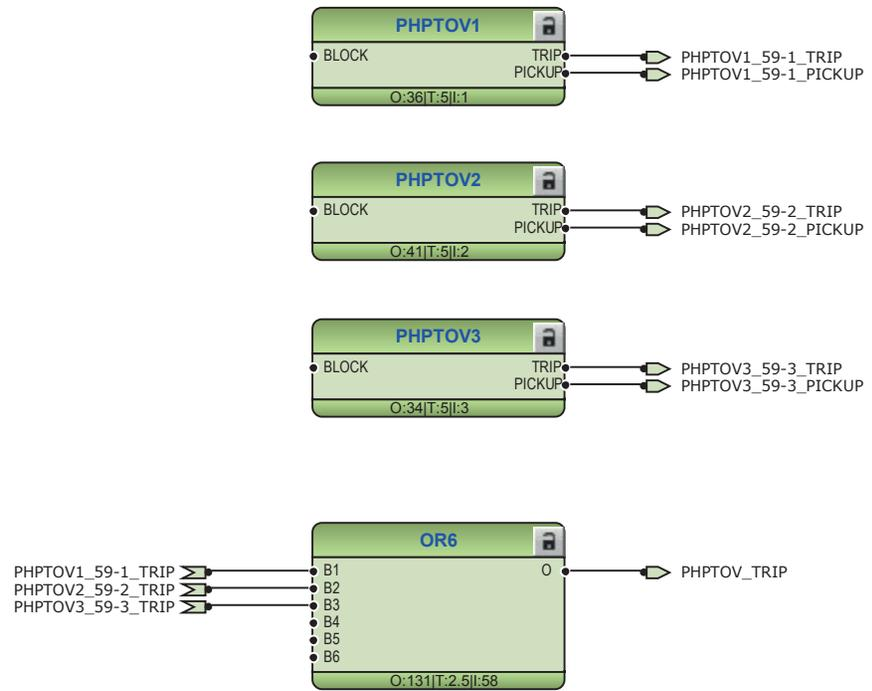
Figure 182: Overvoltage protection function
