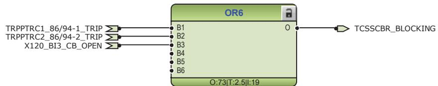
Figure 33: Logic for blocking of trip circuit supervision
