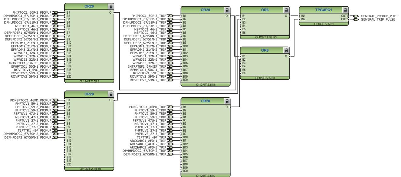
Figure 188: General pickup and trip signals
