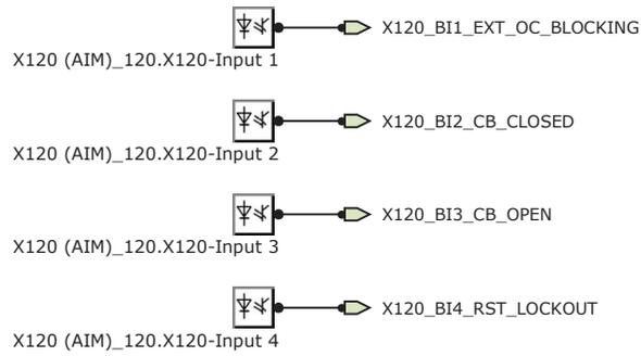
Figure 102: Default binary inputs - X120
