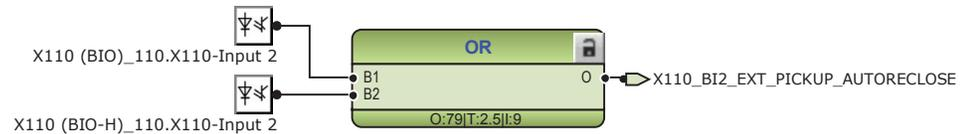
Figure 215: Default binary inputs - X110
