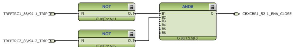
Figure 86: Circuit breaker close enable logic
