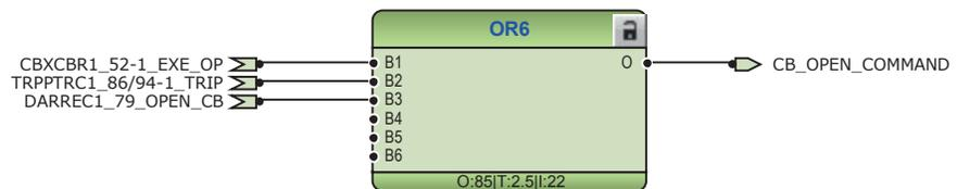
Figure 144: Circuit breaker control logic: Signals for the opening coil of circuit breaker 1
