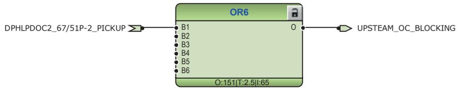
Figure 111: Upstream blocking logic
