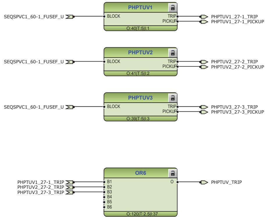
Figure 68: Undervoltage protection function
