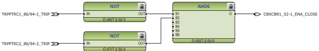
Figure 37: Circuit breaker close enable logic
