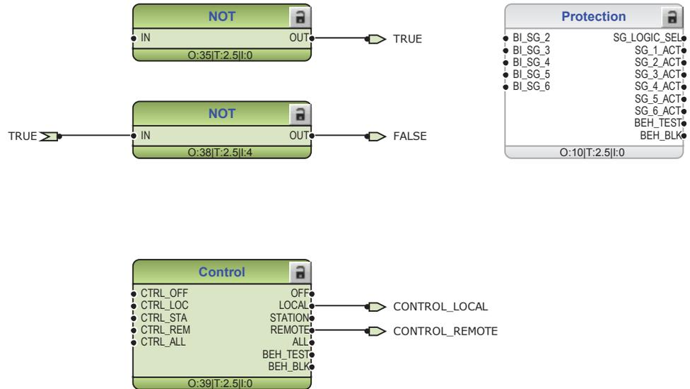
Figure 49: Functions for general logic states TRUE and FALSE, protection setting group selection and local and remote control
