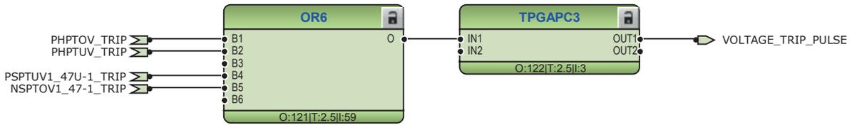
Figure 164: Timer logic for voltage trip and frequency protection trip alarm
