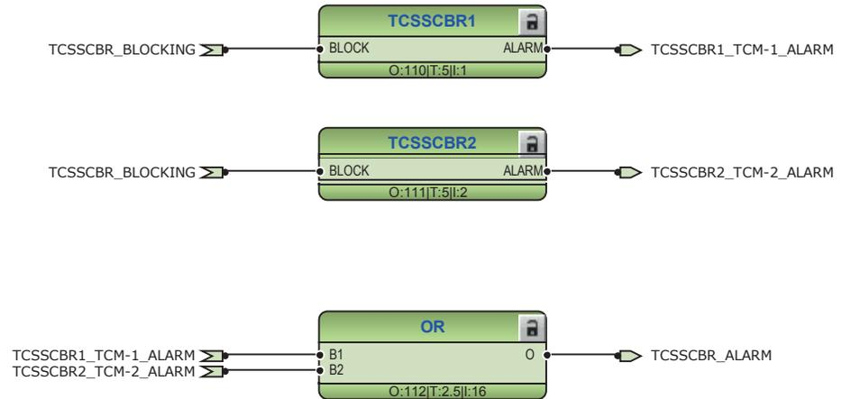
Figure 139: Trip circuit supervision function
