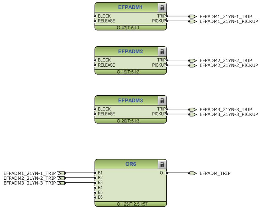
Figure 61: Admittance-based ground-fault protection function
