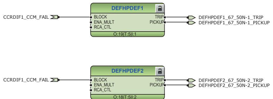
Figure 229: Directional calculated neutral overcurrent protections
