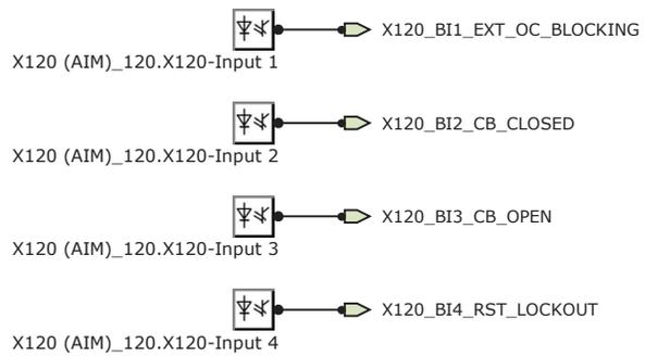
Figure 47: Default binary inputs - X120
