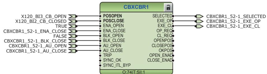
Figure 199: Circuit breaker control logic: Circuit breaker 1
