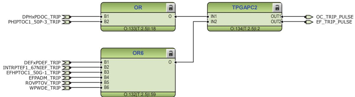
Figure 105: Timer logic for overcurrent and ground-fault trip pulse
