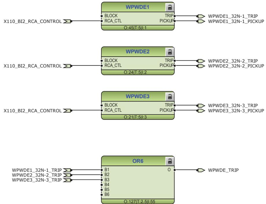
Figure 60: Wattmetric protection function
