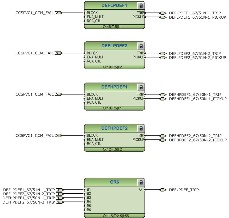
Figure 172: Directional ground-fault protection function
