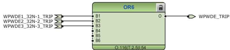
Figure 175: Wattmetric protection function
