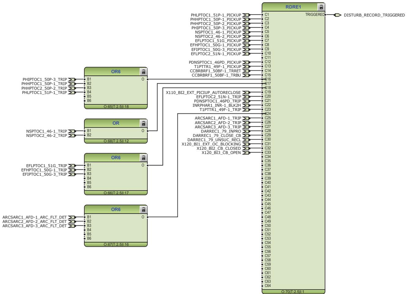
Figure 29: Disturbance recorder
