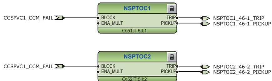
Figure 171: Negative-sequence overcurrent protection function
