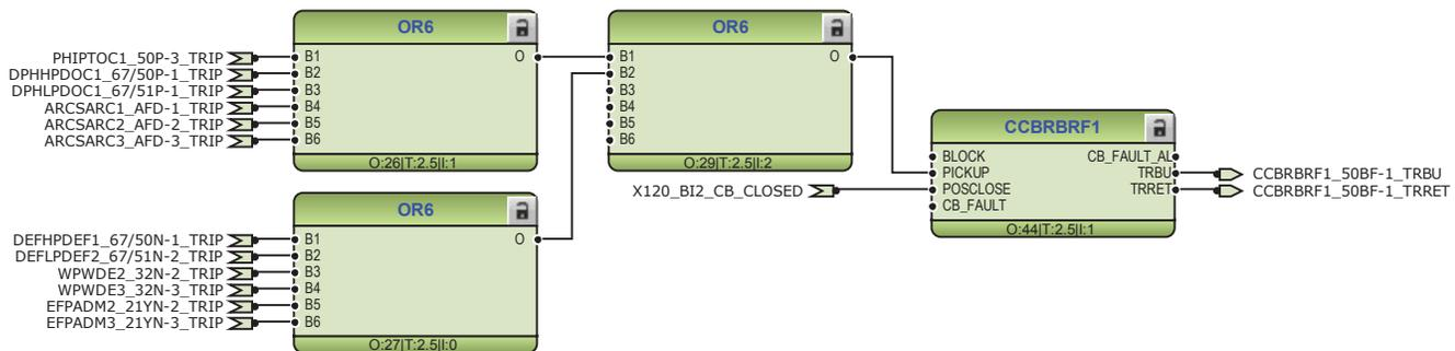
Figure 64: Circuit breaker failure protection function
