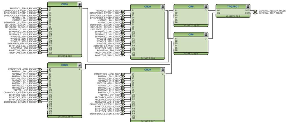
Figure 130: General pickup and trip signals
