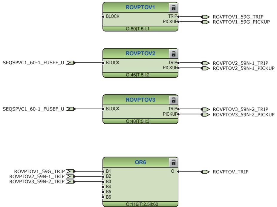
Figure 128: Residual voltage protection function
