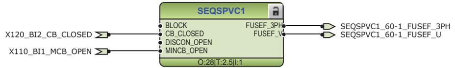
Figure 78: Fuse failure supervision function
