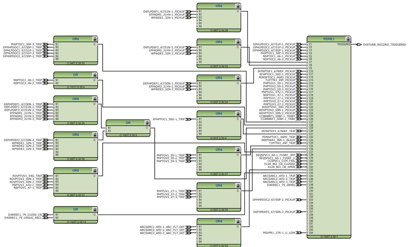
Figure 192: Disturbance recorder
