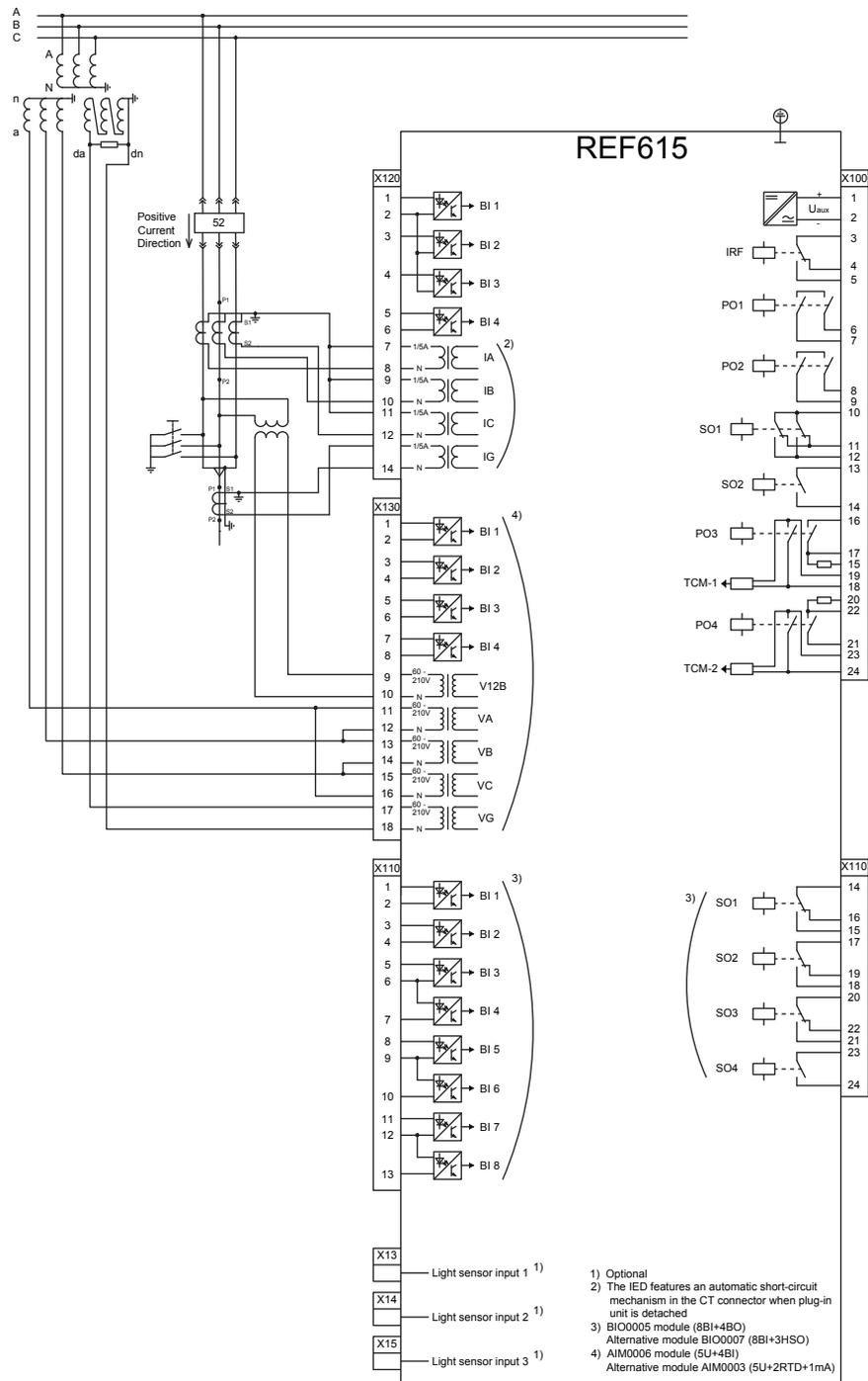
Figure 12: Connection diagram for the N configuration
