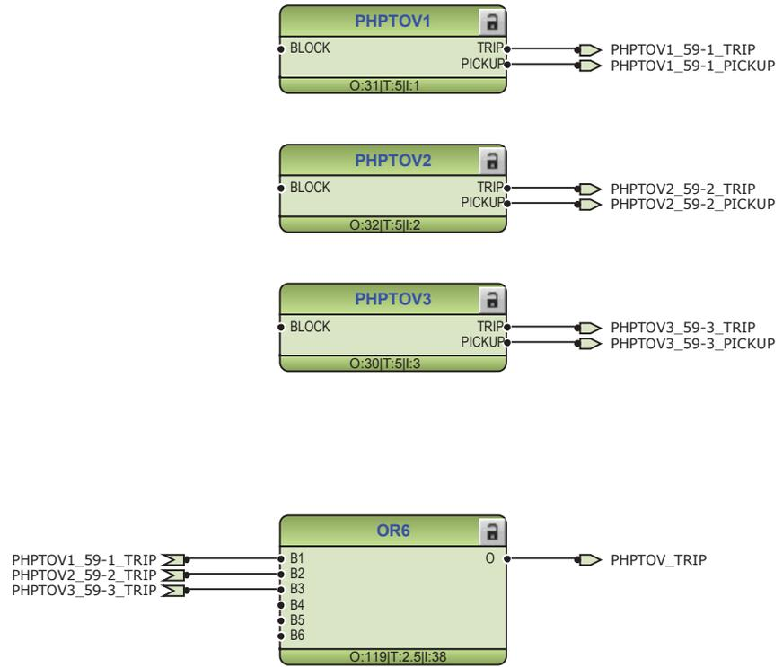
Figure 67: Overvoltage protection function
