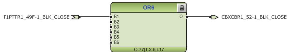
Figure 89: Circuit breaker 1 close blocking logic
