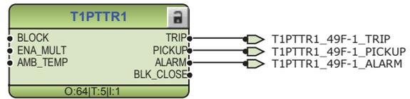
Figure 21: Thermal overcurrent protection function
