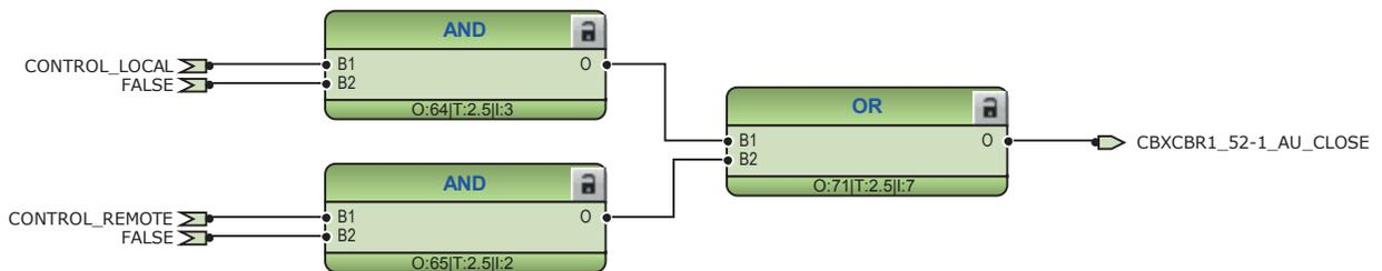
Figure 203: External closing command for circuit breaker
