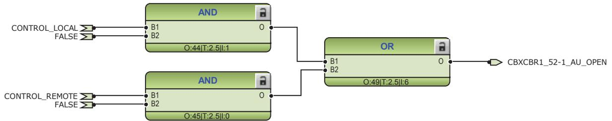
Figure 39: External opening command for circuit breaker
