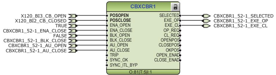
Figure 83: Circuit breaker control logic: Circuit breaker 1
