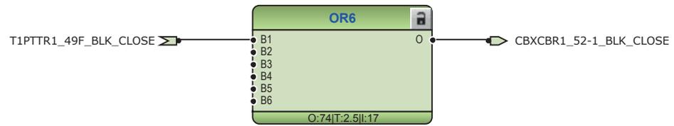
Figure 146: Circuit breaker close blocking logic
