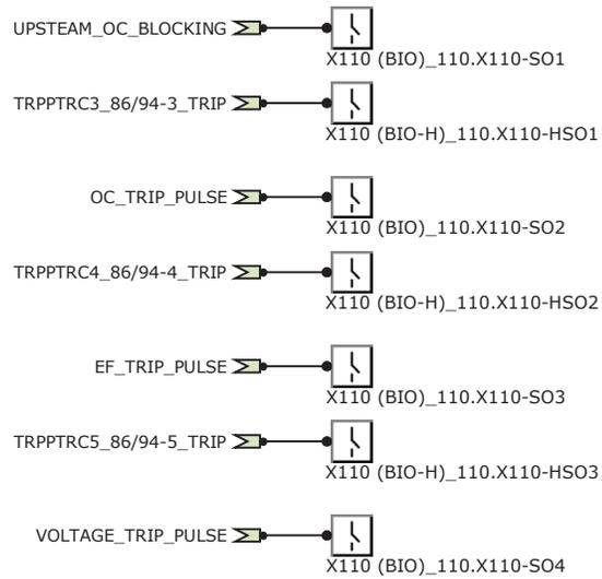
Figure 159: Default binary outputs - X110 terminal block
