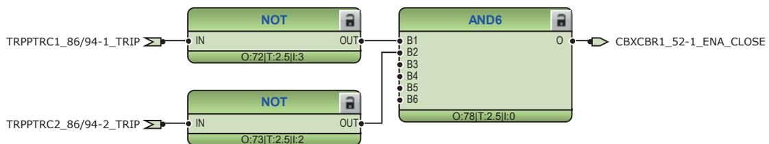
Figure 145: Circuit breaker close enable logic
