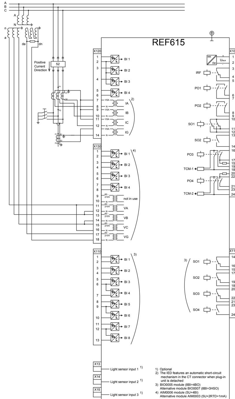
Figure 10: Connection diagram for the F configuration
