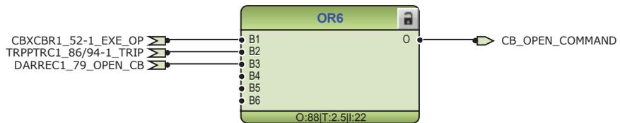
Figure 85: Circuit breaker control logic: Signals for the opening coil of circuit breaker 1
