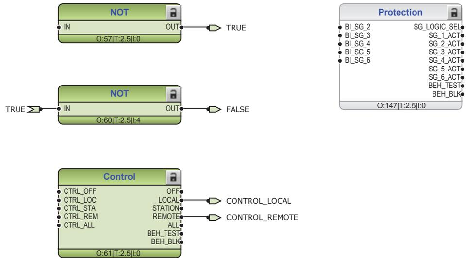
Figure 220: Functions for general logic states TRUE and FALSE, protection setting group selection and local and remote control
