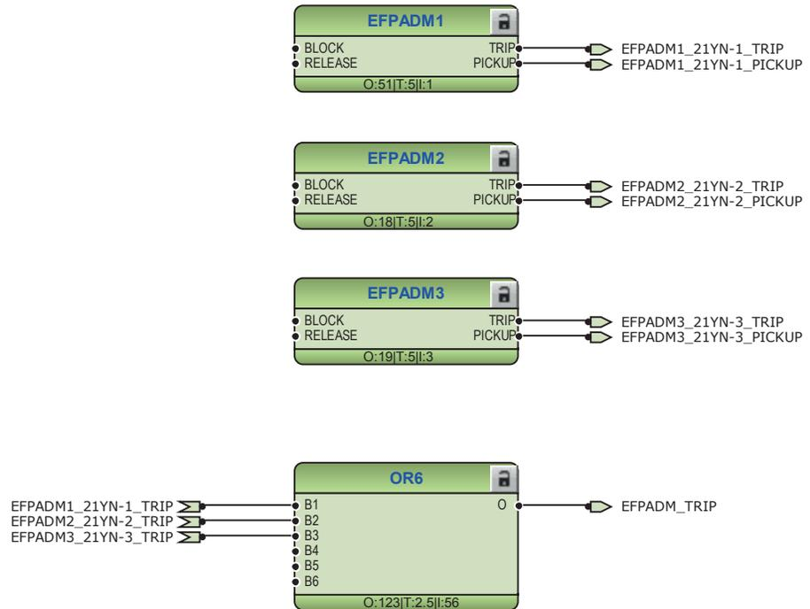
Figure 118: Admittance-based ground-fault protection function
