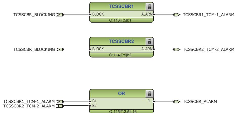
Figure 81: Trip circuit supervision function
