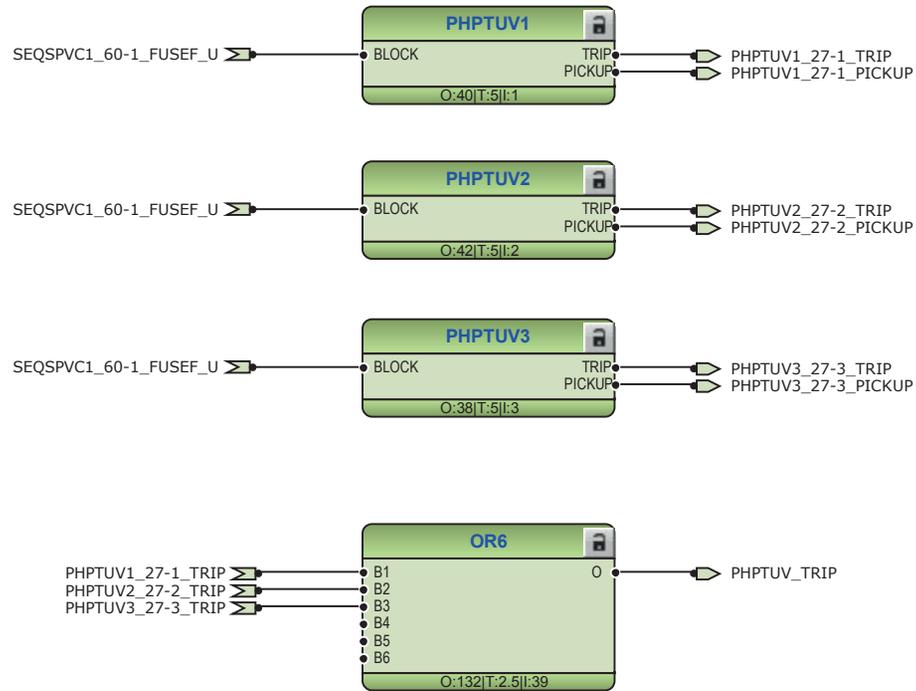
Figure 183: Undervoltage protection function
