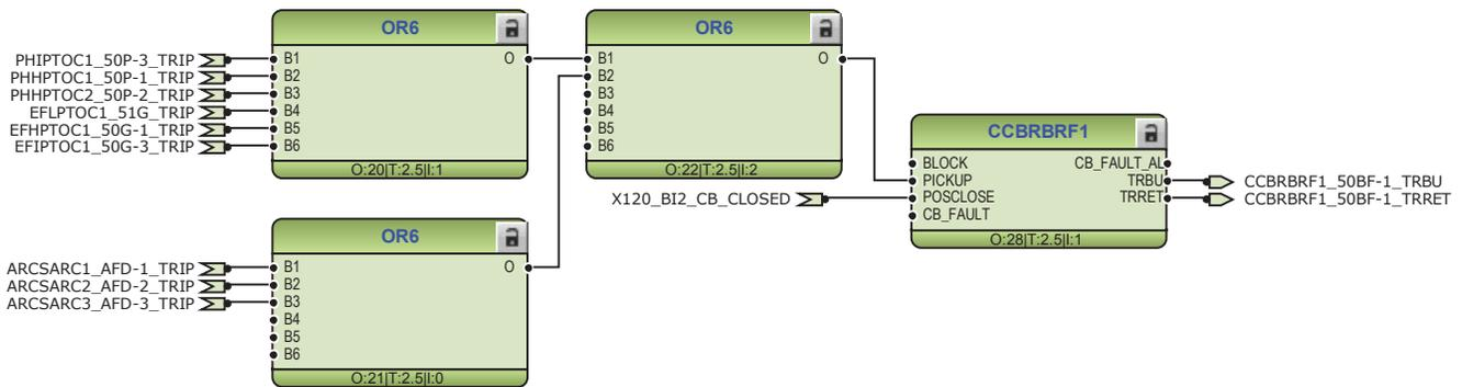
Figure 22: Circuit breaker failure protection function
