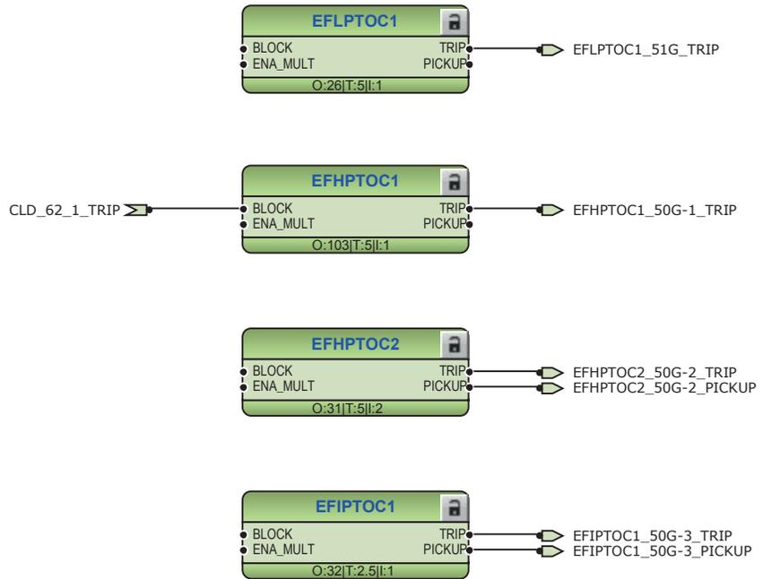
Figure 228: Non-directional ground-fault protection
