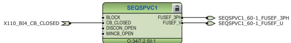
Figure 136: Fuse failure supervision function
