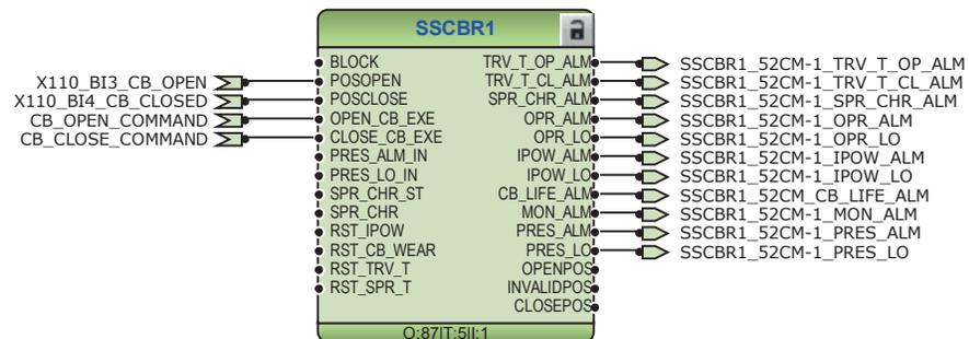
Figure 137: Circuit-breaker condition monitoring function
