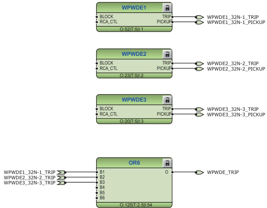
Figure 117: Wattmetric protection function
