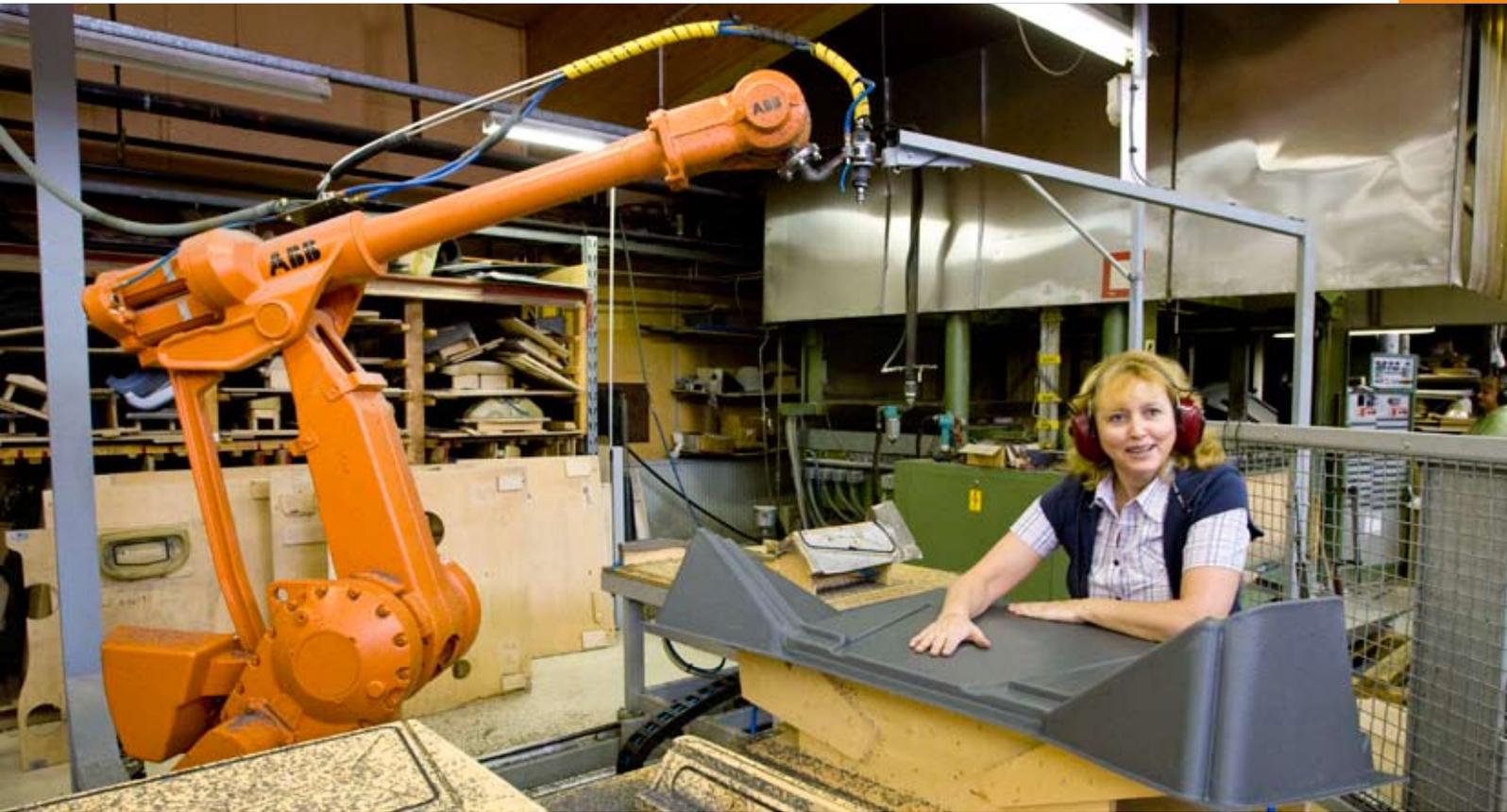
**Finnish company Volar Plastic uses robots for sawing or waterjet cutting plastic parts for the tractor and forestry machine industries. And software that allows for offline programming gives the company an edge over its competitors.**
