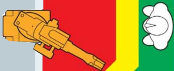
SafeMove confines the robot motion to safe zones, allowing for safe closer interaction between operator and robot.
