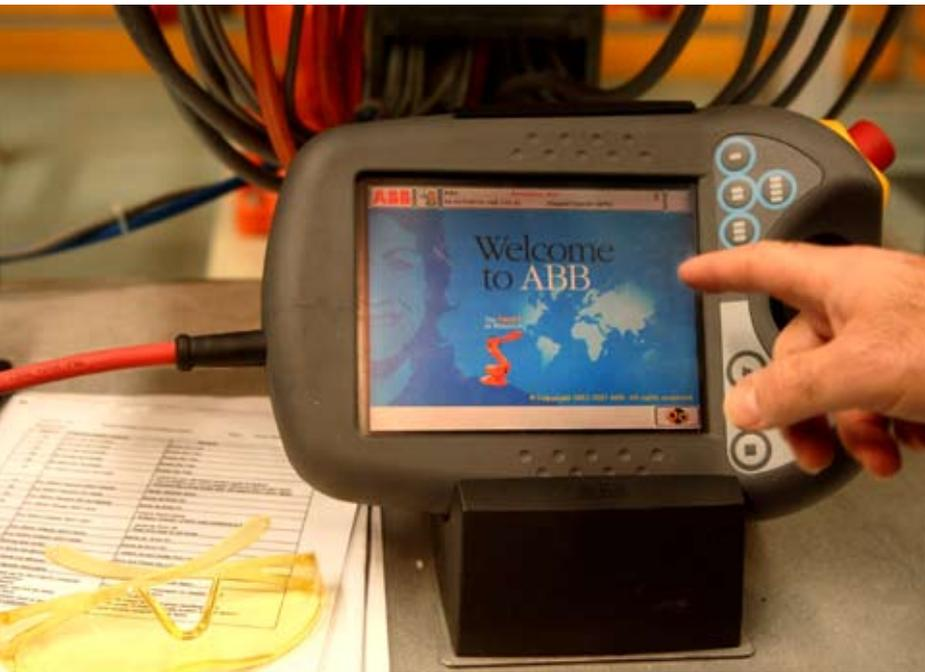
The FlexPendant of the IRC 5 robot controller is part of the user-friendly system that includes an IRB 4400 robot.
