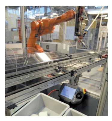
According to Persson, the line is capable of assembling one fuse switch disconnector per minute and has substantially increased Kabeldon's productivity. Previous assembly was done manually at four different workstations, which obviously took more time and required more floor space. "Another benefit is that the quality of the units has noticeably improved," says Persson.
