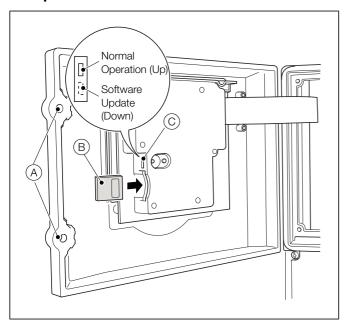
Fig. 3.1 SD Card Removal
