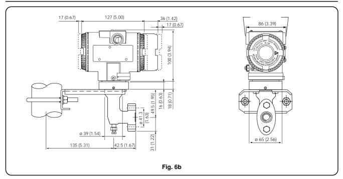
Adapter angle (90°) entry connection (7/16in – 20 UNF drilling)
