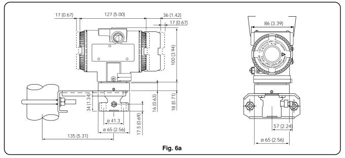
Adapter straight (180°) entry connection (7/16in – 20 UNF drilling)
