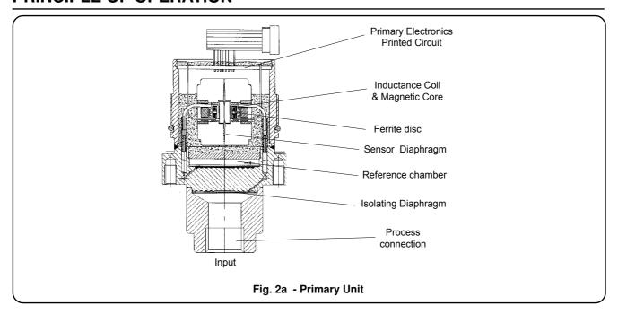
The instrument consists of two functional units:
