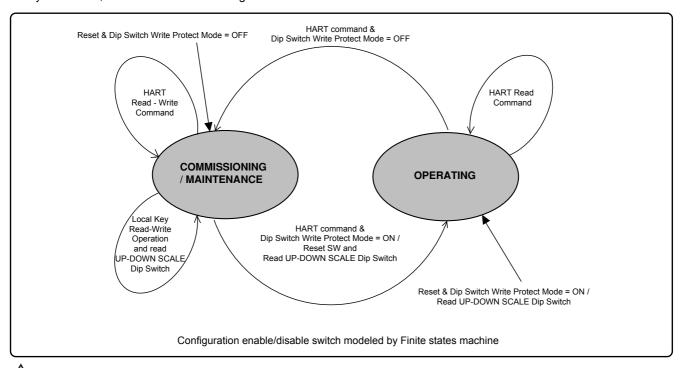
WARNING - The transmitter is considered in safety condition (normal operating mode) when the switch is in Write Protect (off). In that condition only reading commands are enabled.
