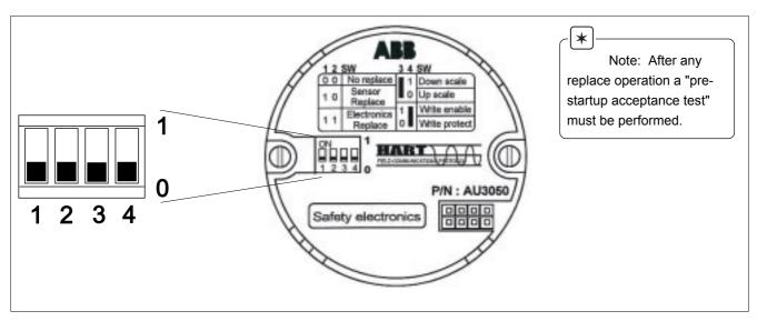
Switches 1 and 2 are used for Electronics or Transducer replace; Switch8 is for Write Protect mode selection; Switch4 is for Up/ Down Scale selection. Here below a description of the operations.
