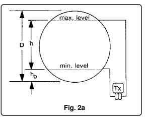
If it is required the partial volume starting from (i.e. the volume at  $h_0 = 0$ ) then the Accoefficient should be equal to the polynomium solved for  $h_0$  with negative sign: for example for  $h_0 = 20\%$
