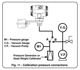
Note that calibration accuracy is strictly related to the accuracy of the test equipment: the use of a dead weight tester is highly recommended.
