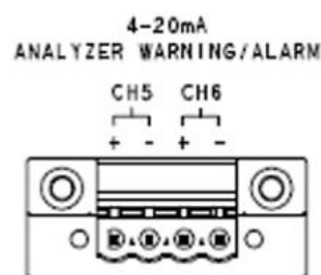
Fig. 69 Gas Analyzer Warning/Alarm Phoenix Connection Points
