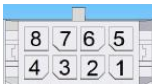
Fig. 123 J2 Connector Pinout
