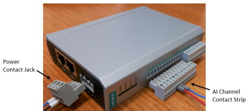
Fig. 63 Modbus Power & AI Connection Points
