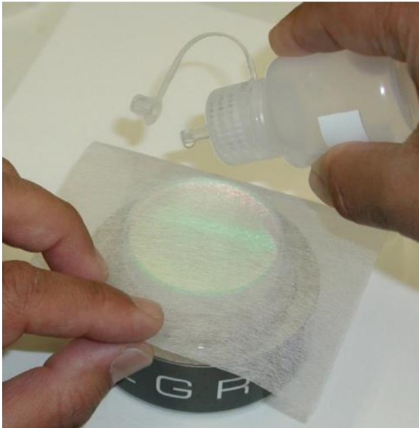
Fig. 101 Where to Apply Cleaning Solution on Lens Tissue
