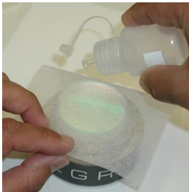
Fig. 135 Where to Apply Cleaning Solution on Lens Tissue
