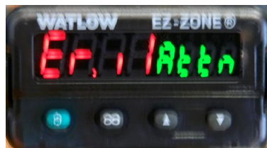
Fig. 73 Temperature Controller Error: Missing Thermocouple Signal
