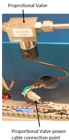
Fig. 114 Proportional Valve Power Connector
