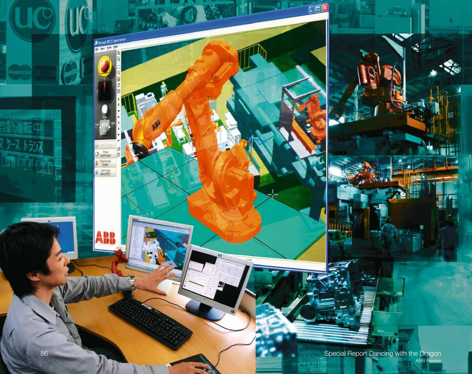
Conventional robot simulation and offline programming tools are usually designed for skilled engineers rather than for sales personnel whose engineering background may be limited. From a salesperson's point of view, existing simulation and offline programming tools are difficult to use. They require knowledge of geometric modeling, the ability to generate and adjust robot targets and paths, perform path configuration, position cell objects and so on.
