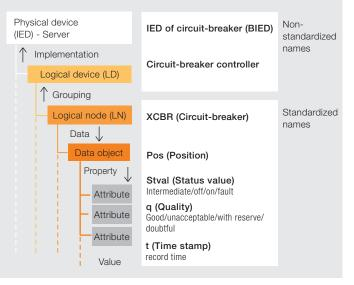
The IEC 61850 object-oriented data model of a physical device
