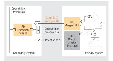
Process bus with "merging" unit (MU), circuit-breaker interface (BIED) and external Ethernet switch
