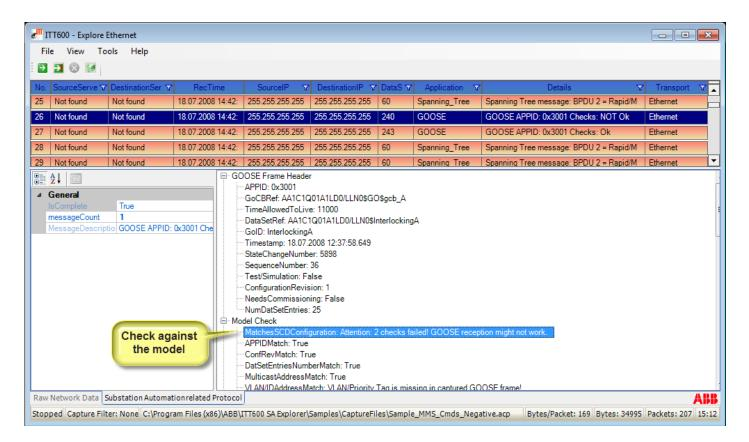
Another method for supporting the distributed function test is provided by a time trend of GOOSE messages between IED, which allows interaction between various applications such as interlocks to be easily monitored.
