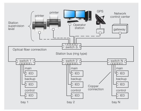
Example of non-redundant station bus
