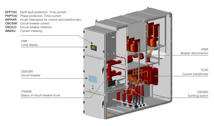
The data model for a medium voltage switchgear unit
