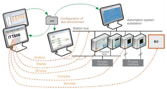
The tool can be connnected to both the system bus and directly to an IED.
