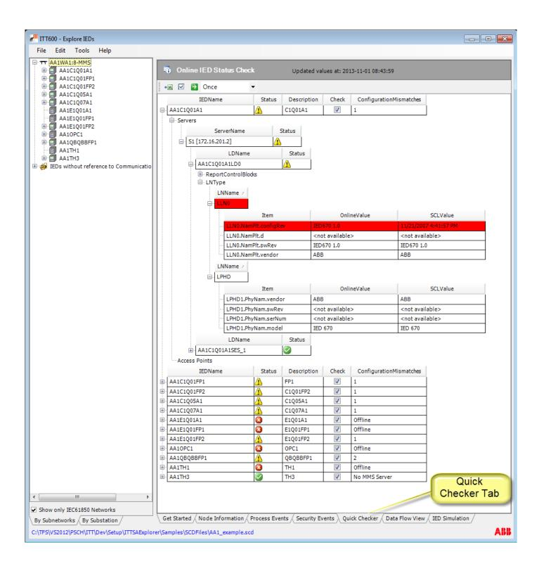
In a similar way, decoding of GOOSE messages by means of the ITT600 SA Explorer tool with clear texts, information about the application and relative mapping in the SCD file, provides an excellent view of Ethernet traffic.
