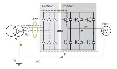
type A (for single-phase UPS) when the UPS project contemplates the possibility of an earth fault current with direct current components.
