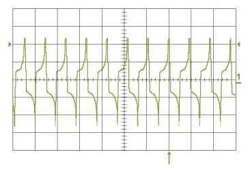
A resistance in series with the winding creates a voltage drop, whose value is sent to a microprocessor including a low-pass filter.
