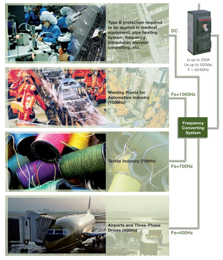
The following table shows some typical applications with power electronics, where type B residual current devices can be used; in particular, they are necessary in the examples 2-36-7 because of the predominant presence of the direct component which could not be detected by type A-AC residual current devices.
