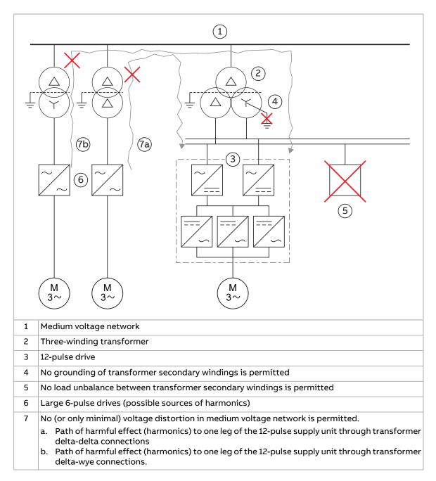
Use identical supply cables between the transformer secondary windings and the drive (type, size, length, quantity).
