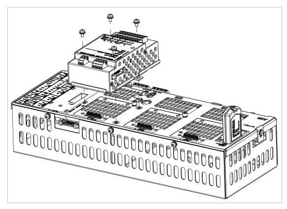
4. Torque the FSO module electronics grounding screw to 0.8 N·m (7.1 lbf·in).
