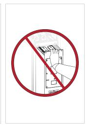
Be careful when handling a tall module. The module overturns easily because
