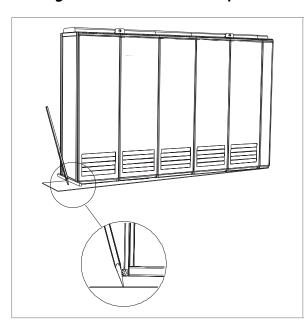
Move the cabinet into its final position with a slate bar (spud bar). Put a piece of wood between the edge of the cabinet and the bar to protect the cabinet frame.
