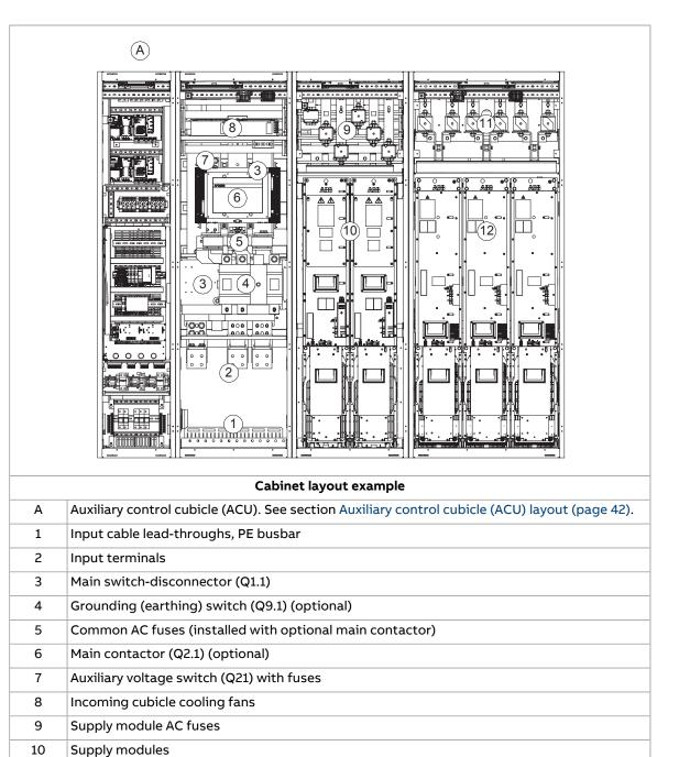
Inverter modules. The output terminals are located behind each module. Each module must be individually connected to the motor using separate cables unless the drive is equipped with option +H359 (common motor terminal cubicle) or +H366 (common output terminals).
