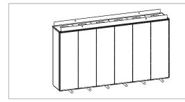
Lay the cabinet on the rollers and move it carefully until close to its final location.
