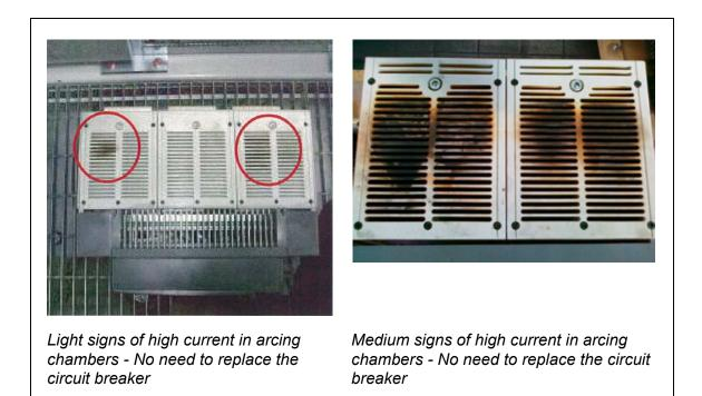
If any of the top grid area of the arching chambers is fully covered with brown/black marks or if there is any sign of black soot on the breakers body or rear terminals, the breaker must be replaced at once and sent for workshop checking. See the example in the figure below.
