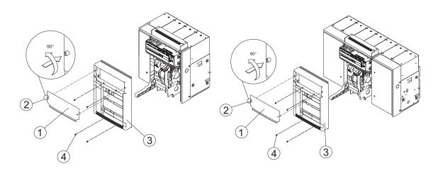
• If the undervoltage coil is installed, disassemble the coil support and relieve the springs of the operating mechanism by closing and opening the circuit breaker.
