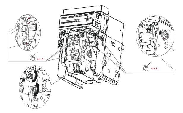
• In case of deformed or oxidized springs, safety rings out of place, or hard wear of operating mechanism, contact ABB SACE. ABB may replace spare parts type A after having obtained the customer's approval.
