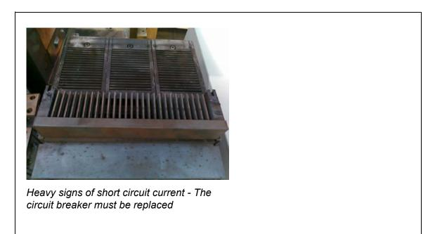
Before actual next trial, check the power cabinet and the converter visually that there are no signs of short circuit or arc. Check especially the following locations:
