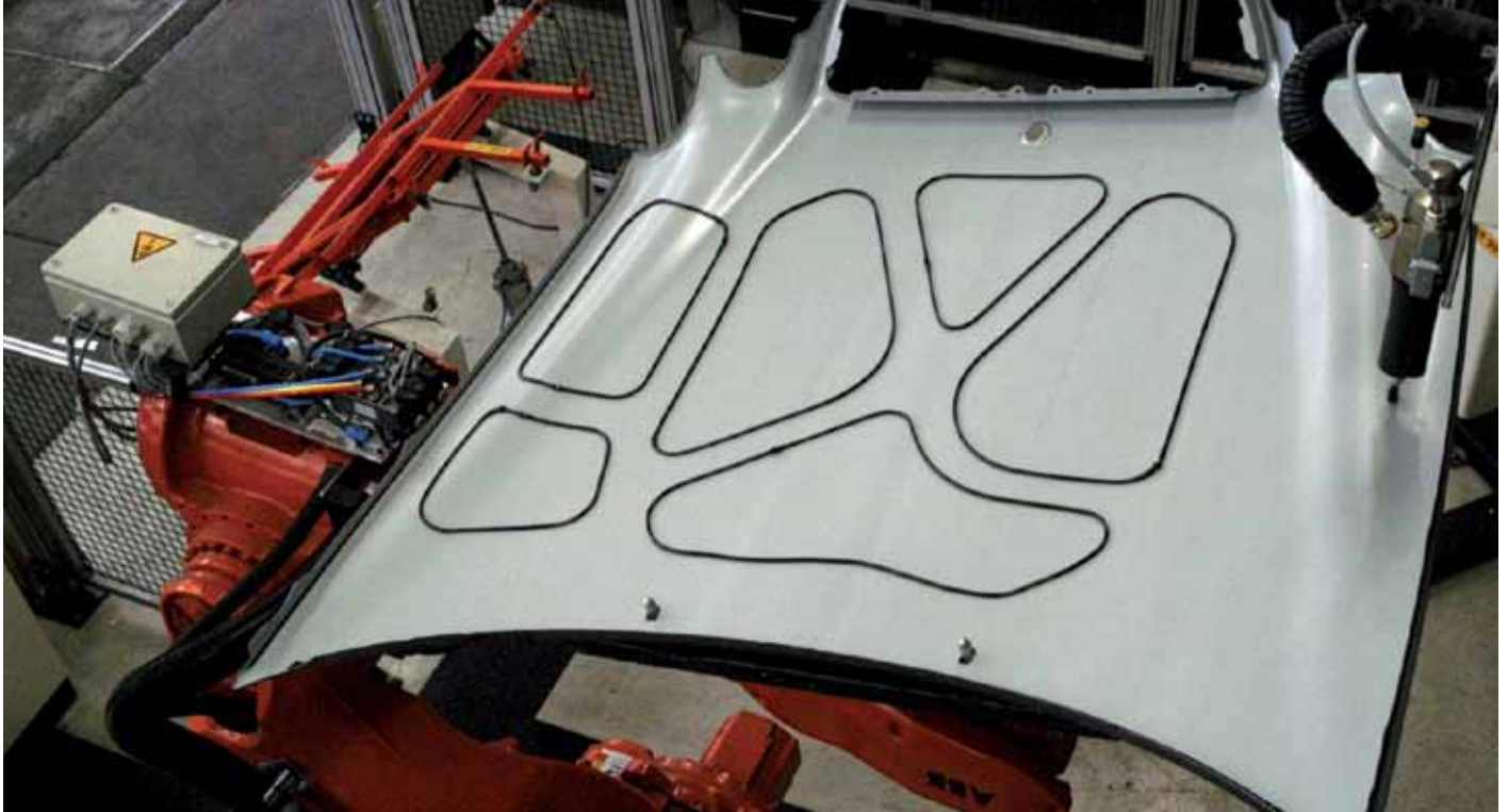
Robot gluing a hood to a Mercedes CLKC208.
