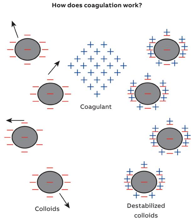
Figure 4 The coagulation process
