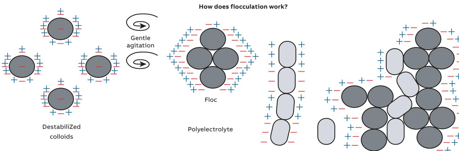
Figure 5 The flocculation process
