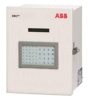
This new generation of flow computers and RTUs offers a low-power, high-reliable microprocessor-based unit with a new Linux operating system, persistent memory, and new connectivity, combined with the same wide range of measurement, monitoring, and alarm applications for remote oil and gas systems. It also provides an upgrade path to new digital technologies and protocols such as MQTT, and a secured wireless connection (WiFi-Access Point or Bluetooth).
