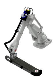
The benefits of traditional robot automation are enhanced by the addition of a rotational 7th axis. Thanks to the 7th axis, the robot keeps the orientation of the part when transferring it from the press to the next. This entails lower inside-press time occupation and better overlapping between loading and unloading robots.
