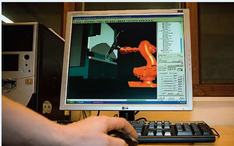
The graphic interface of Press Brake Tending ProcessPac adds to the ease with which the operator can program and simulate the robot cycle.
