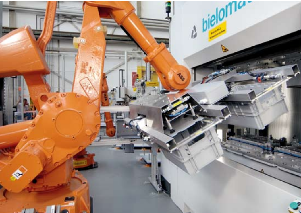
There are three functions for robot No. 3: labelling, checking and stacking.
