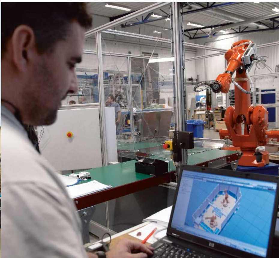
Anders Hedström of Specma AVT uses ABB Robot Studio software on a PC to program robots offline.
