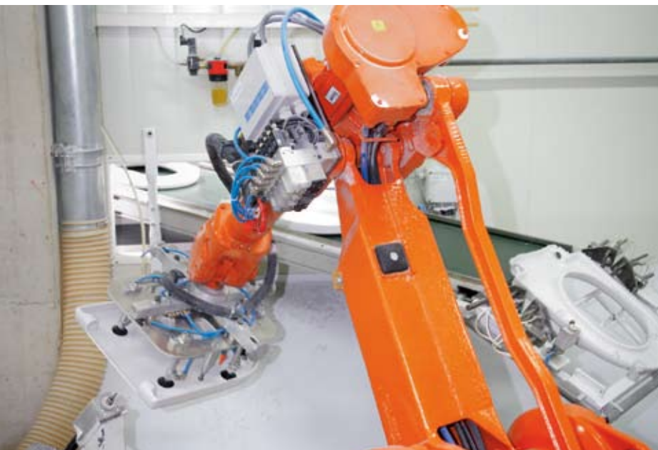
The IRB 2400 robots can be reprogrammed for a new toilet seat model in only 15 minutes.
