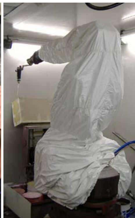
Ranger Production Manager GianLuca Ceppi and Maintenance Manager Diego Zotti; at right, an IRB 5400-12 paint robot works applying enamel for Italian and German automobiles.
