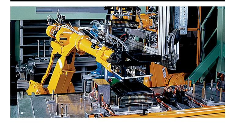
A new automating concept makes it possible for automobile supplier Seeber to equip micro filter housing after injection moulding with several seals fully automatically. Compared to conventional sealing processes, direct application of sealing agents onto the housing with EDF mixing and dosing systems in connection with an ABB robot saves money and increases flexibility.
