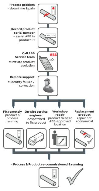
Figure 1 Technical support and corrective maintenance flowchart
