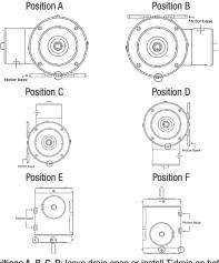
Positions A, B, C, D: leave drain open or install T'drain on both ends of the motor at circuled locations. Plug all other drain holes. Positions E, F: leave drain open or install T'drain at circled locations. Plug all other drain holes.
