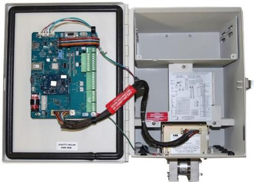
Figure 1-2: XRC<sup>G5</sup> inside the enclosure
