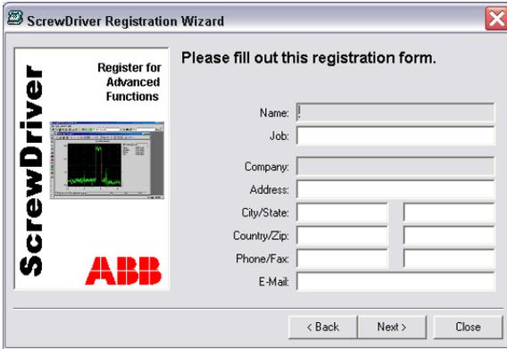
**Note.** The *Name:* and *Company:* fields are completed automatically and cannot be changed. The remaining fields must all be completed for registration to be successful.
