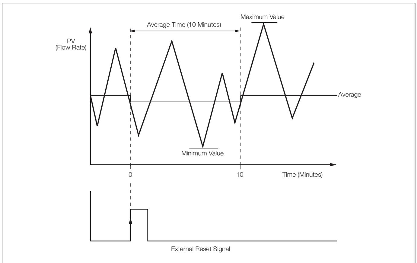
Fig. 2.1 Example of Average, Maximum and Minimum Functions
