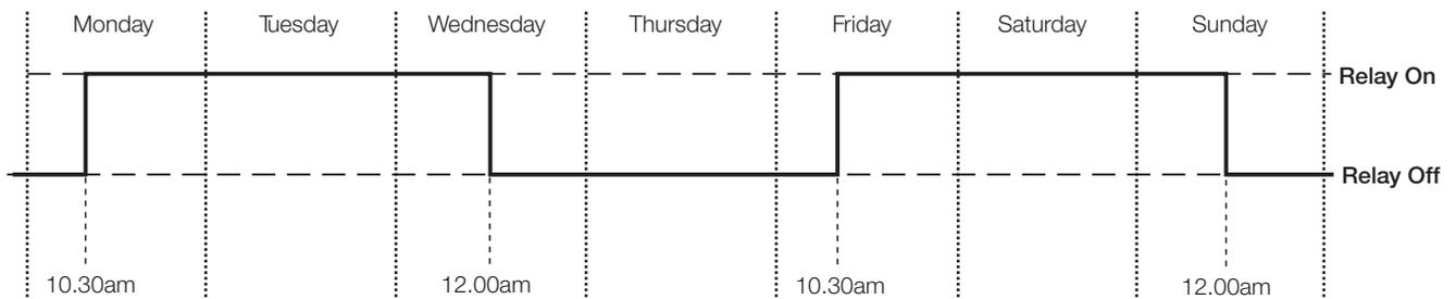
**Example A** – shows timer option programmed to energize relay output for 49 hours 30 minutes over a two day period
