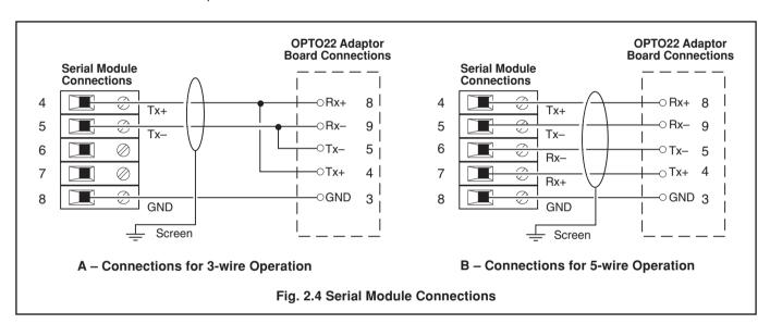
**OPTO22 Board Pin Identification COMMANDER 1900 Serial Module Terminal Board Terminal Number** Connections Part Number AC24 AT & AC34 Connections TX+ 4 TX+ 4 8 RX+ TX-5 5 TX-9 RX-**GND GND** 8
