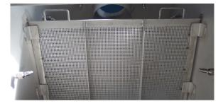
After the cleaning, the drainage of the filter is triggered by the opening of an automatic valve at the bottom of the filter. Accumulated solids and contaminants flow out the bottom drain nozzle to the sewer. A tangential water inlet nozzle helps to flush the solids remaining on the bottom surface in order to completly clean the filter.
