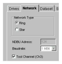
If the check box is not selected, the module will write the fieldbus configuration parameters and start controlling the drive. This will interfere the R-series adapter, which will loose its configuration and capabilities for control.
