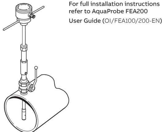
Figure 6 Typical installation (metal pipe)
