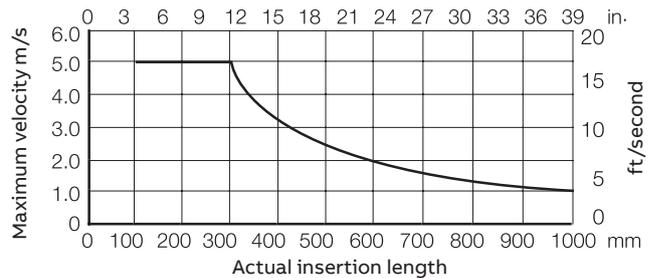
Figure 7 Maximum allowable velocity for different insertion lengths
