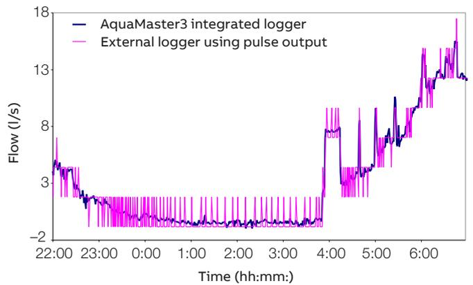
Figure 4 Elimination of pulse quantization with AquaMaster3
