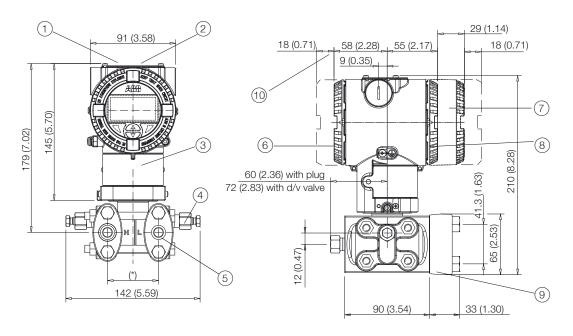
$54\ (2.13)\ mm.\ (in.)\ on\ 1/4\ in.-18\ NPT\ process\ flange\\ 51\ (2.01),\ 54\ (2.13)\ or\ 57\ (2.24)\ mm.\ (in.)\ according\ to\ 1/2\ in.-14\ NPT\ adapters\ fitting;$ (\*)
