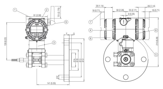
1 Adjustments | 2 Identification plate | 3 Certification plate | 4 Terminal side | 5 L1 and L5 integral display housing | 6 Electronic side | 7 Space for cover removal | 8 Battery housing of WirelessHART version | 9 Antenna of WirelessHART version
