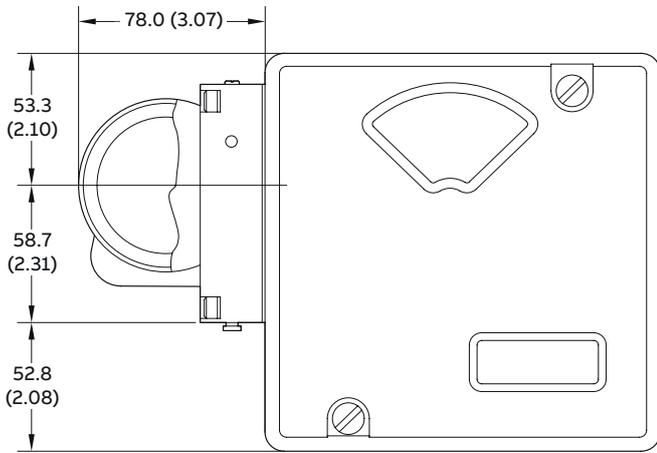
Figure 7 View with explosion proof I/P converter
