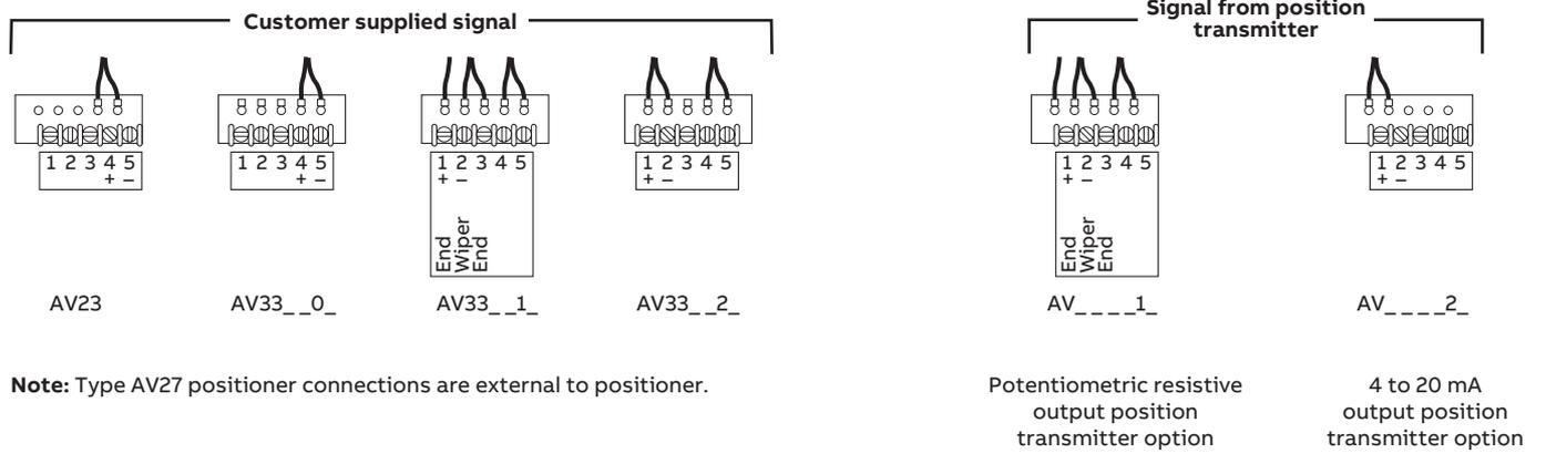
Figure 13 Signal input and output connections
