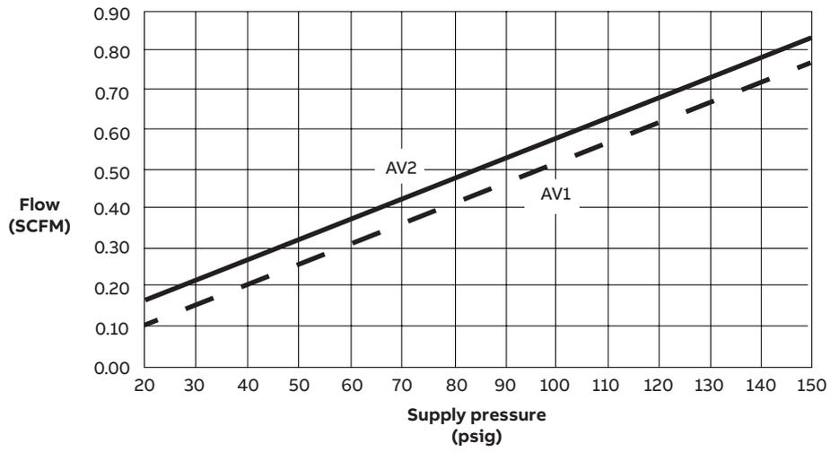
Figure 1 Air consumption (at null)
