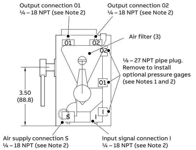
Figure 9 View with optional manifold
