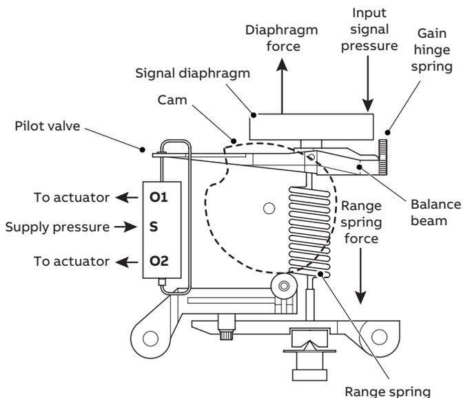
Figure 3 Operation diagram
