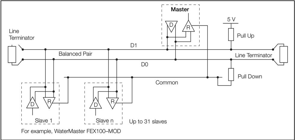
Fig. 2.1 Typical MODBUS RS485 2-Wire Network Installation
