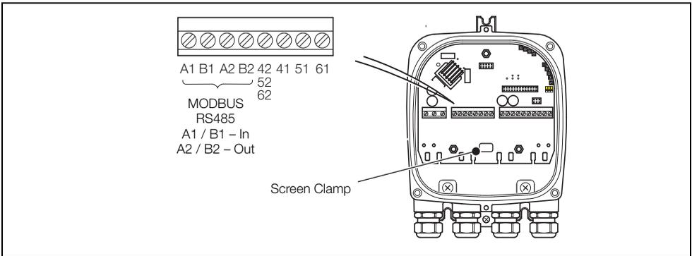
Fig. 3.1 WaterMaster FEX100-MB RS485 Backplane Wiring Terminal Connections to MODBUS Network
