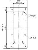
To fill up the corner between two coupled enclosures
