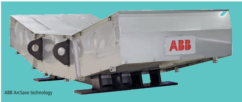
hardware is installed under the furnace bottom – but not in contact with it – and generates a travelling electromagnetic field that penetrates into the furnace and generates a magnetic force within the melt that produces the stirring effect. This results in improved mass and heat transfer through the melt.
