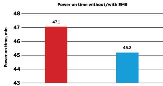
Effect of ArcSave® on electric energy consumption (left) and power on time (right) reduction
