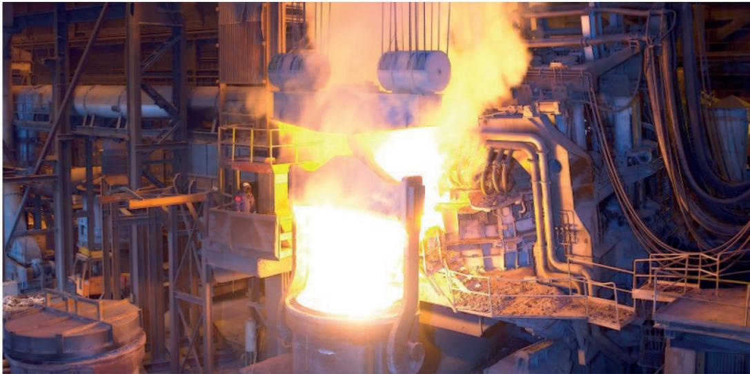
Electric Arc Furnace in operation
