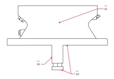
01 - The load bearing is in the ODE end plate to protect it from the heat
