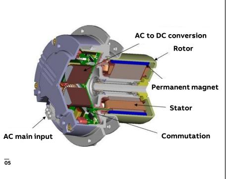
EC motors have an AC/DC conversion with a rectifier built-in
