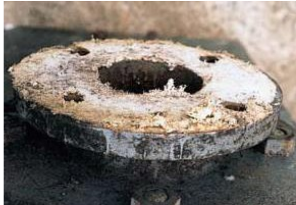
Remains of Asbestos (of flange gasket)
