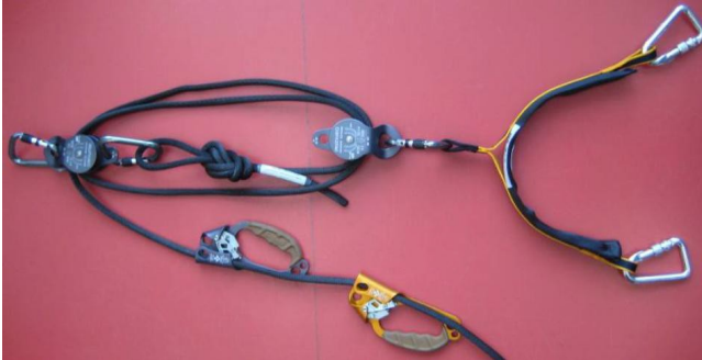
Figure 23.2: Example of pre-assembled lifting equipment, ready to use in emergency
