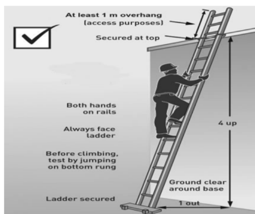
Figure 15.2: Correct set-up of ladder
