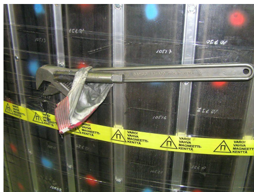
Ferromagnetic tools cause real danger
