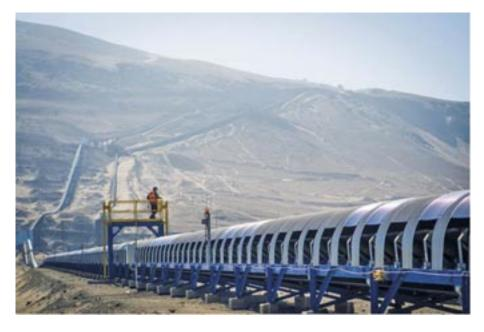
gearless motors; and an 1,830 mm wide, 1,043 m long overland conveyor #2 powered by head and tail end 550 kW VFD driven motors. Siemens supplied the complete electrical solution to thyssenkrupp. The EP project was awarded in 2014 and began operations in late 2017. Elsewhere on the current projects, for Oyu Tolgoi Siemens is suppling the gearless drives for the underground conveyor that feed a mine hoist (Phase 1) and the three incline conveyors for Phase 2.
