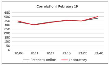
L&W Freeness Online results were regularly compared against laboratory results to ensure accuracy. This example shows the comparison over a two hour period, on two separate days, with nearly identical results.
