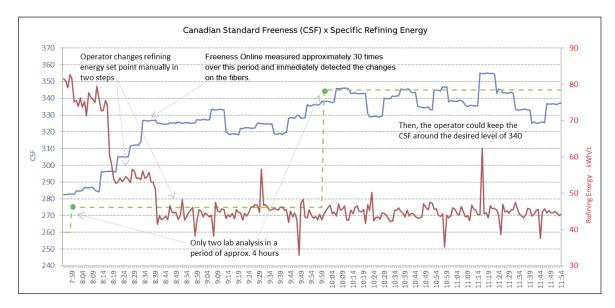
L&W Freeness Online was able to measure every 6-7 minutes – significantly less than the two-hour intervals of the manual test – helping to quickly detect the fiber changes. Without online measurement, the operator could not safely manipulate refining energy and maintain the freeness at target level.
