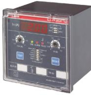
Front panel residual current relays are electronic devices used in combination with an external toroidal transformer. They are according to the protection standard IEC/EN 60947-2 Annex-M. The sensitivity can be set from 0.03 A to 30 A, while the tripping time from 0 to 5 seconds.
