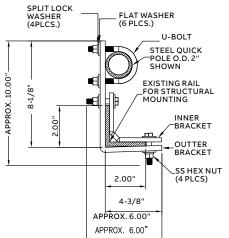
RMB-QP-BKT-N Bracket for structural pole mounting
