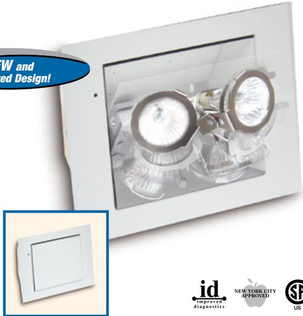
The Phantom Series is architecturally designed for unobtrusive use in walls with cavities (drywalls with 4" studs) or uninsulated ceilings with horizontal beams or T-bar structures. In normal conditions (stand-by), the unit is completely concealed in the wall or ceiling. In case of power failure, the door of the unit rotates open 180° and exposes the emergency lights (two high-efficiency MR16 lamps) to illuminate the path of egress.
