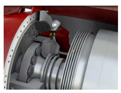
The propeller bearing is of the roller type, but the Azipod unit's shaft thrust bearing is available with both roller and hybrid types depending on the size of the Azipod unit. Hybrid type bearings enable enhanced life cycle cost performance and reliability in icebreaking. Hybrid type thrust bearing pads (to stop wear) can be changed from inside the Azipod unit without dry-docking the ship or pulling out the Azipod module's shaft.
