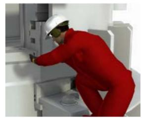
Figure 5-2 Changing the slewing seals from Azipod room without dry-docking (Steering Module 14000)
