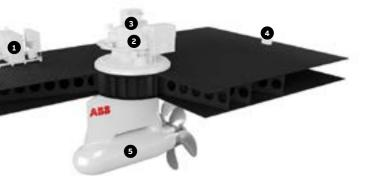
The propeller shaft seal system includes the housing, a combination of a face- and lip-type seal and a liner. The entire Propulsion Module is pressurized, while there are also drainage lines between the face- and lip-type seals.
