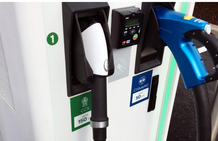
— Widely deployed open charging standards include CCS and CHAdeMO, seen here on Electrify America's network. The CCS standard boasts the highest number of compatible EV makers in North America and Europe.
