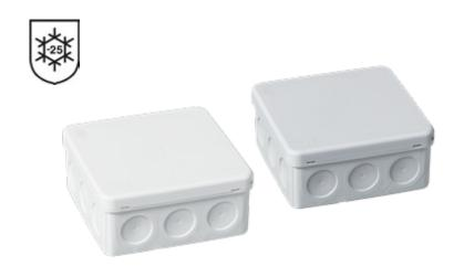
The renewed box includes 14 membrane cable entries (Ø 19 mm): 3 on each sides and 2 at the bottom. The box is approved for IP65 classification and it is protected against cold environment and suitable for use at the temperature down to -25°C.
