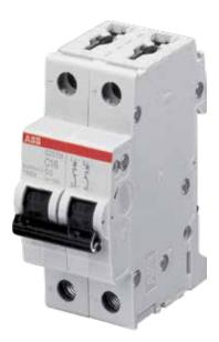
S200 M DC MCB in System pro M compact range impresses with its performance range, approvals and high inbuilt short circuit breaking capacity in DC applications. S200 M DC MCBs can be used in 1-pole version at 220V DC and in 2-pole version up to 440V DC. During the installation process it is necessary to take into account, the polarity marked on the device.
