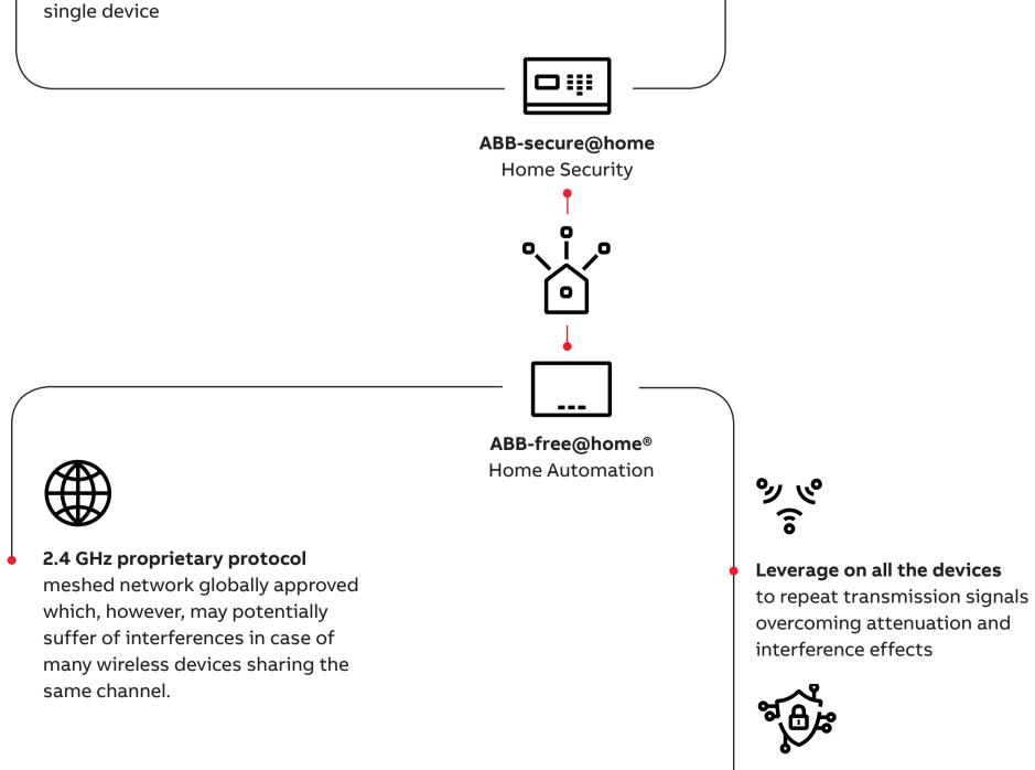
**Digital encrypted communication** at 128 bit
