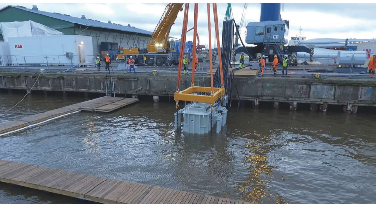
ABB's subsea VSD completed a shallow-water test in 2017. (Source: ABB)
