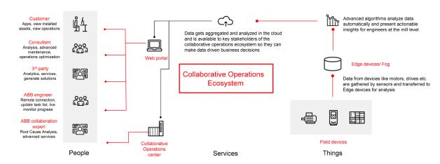
$ABB\ Ability^{\tiny{TM}}\ technology\ collects,\ aggregates,\ analyzes,\ and\ presents\ actionable\ information\ on\ KPIs\ to\ enable\ experts\ to\ improve\ paper\ machine\ performance.$
