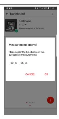
Smart Sensor's measurement interval is set to one hour by default. However, you can change the interval from the asset menu's "Set measurement interval" button to a minimum of 5 minutes.
