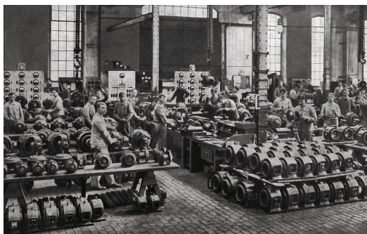
At the beginning of the 20 th century, electric motors began to replace steam engines as the main source of power for machinery. BBC alternating current motors for one-, two- and three-phase current played an important part in this development.
